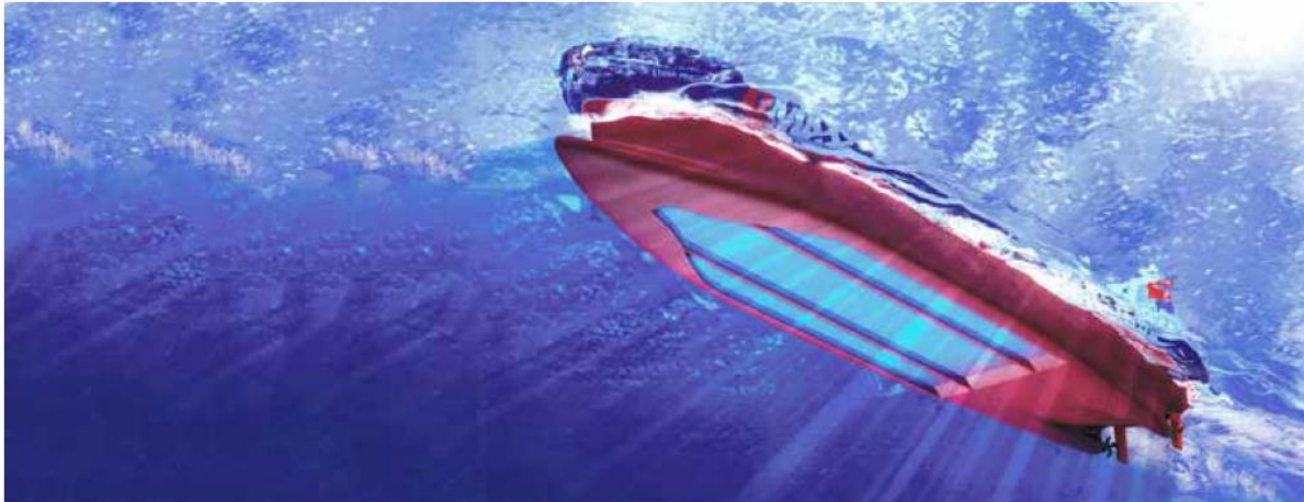
Figure 9: SSPA investigated different designs for the project P-MAX air to minimize the resistance of the 182m tanker. Photo: Courtesy of STENA AB. Read more at www.sspa.se . Air Cavity Illustration [55]
