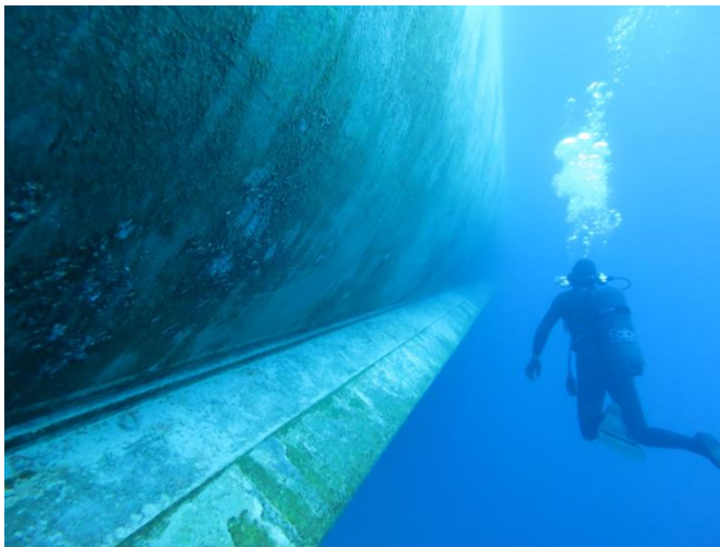
Figure 12: Ship's hull with obvious partial fouling. [22]
