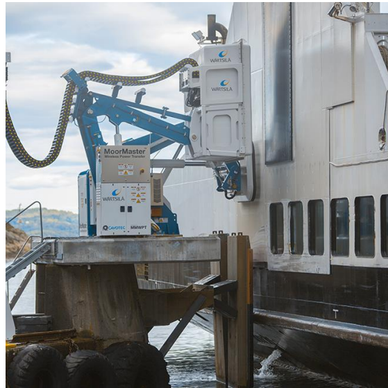
Figure 13: Example of an wireless charging system (wartsilla)
