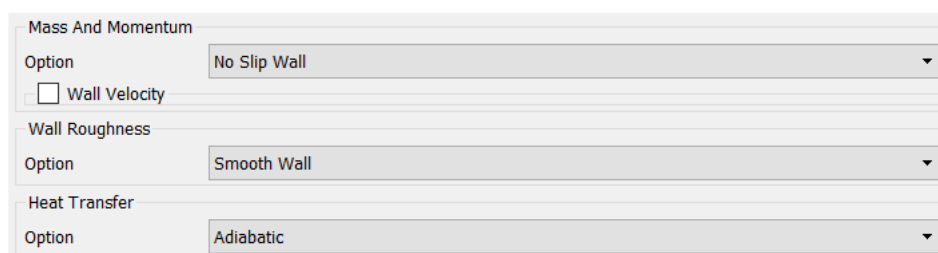
Figure 4.12 Boundary conditions for duct walls.
