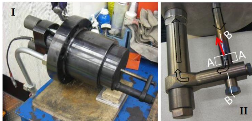
Figure 43 - Assembled injector (I) and view of injector arrangement including flow directions (II) (one-hole fuel injection (red arrow) and redirected bypass-flow (black arrows)) [50].
