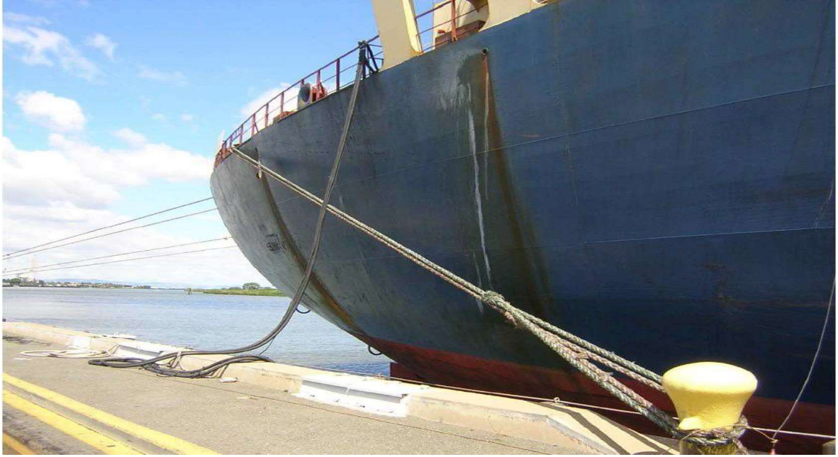
Shore-side power connection at Figure III-8: Shore power connection on the USS POSCO facility in Pittsburg, CA
