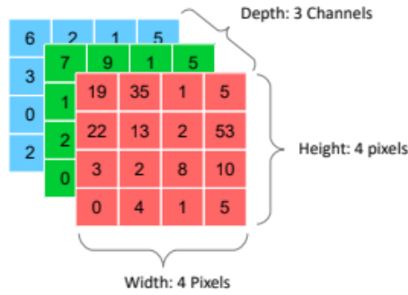
Figure 2.8: Example of an RGB image: A 3D matrix of size 4x4x3
