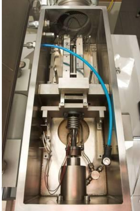
Figure 7.1: The setup of the used dilatometer. The sample is positioned inside the coil and anchored between two metallic rods.
