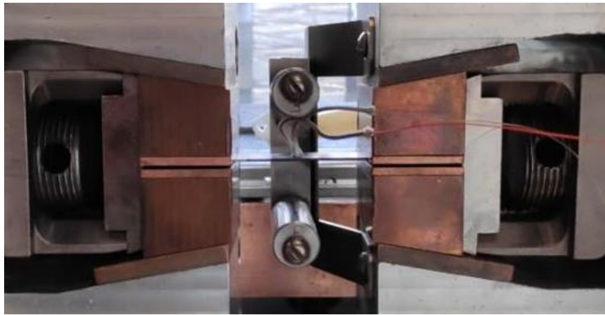
Figure 7.2: The setup of the Gleeble 3800. The sample is anchored between the copper holders and heated by the two coils in the middle of the setup.
