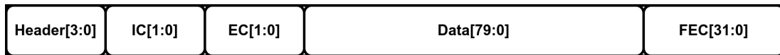
Figure 7.1: Graphical representation of the GBT Frame [63]. The first four bits is the header, then the next four are dedicated fields used for Slow Control, while the Data can be added in an 80-bit field. The FEC field is 32-bit wide, and is used for correcting any errors during the reception of the frame.
