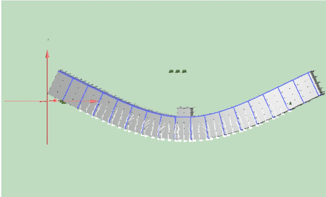
Figure 142. Deformation of the beam in collapse
