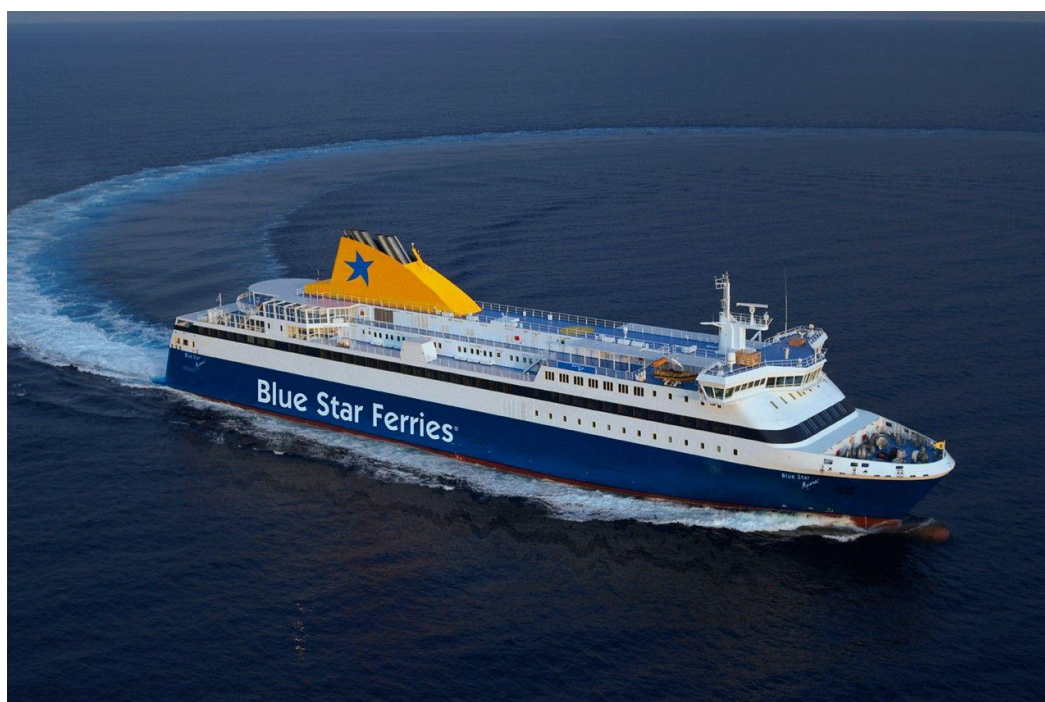
Figure 1-1: Ro-pax ferry Blue Star Myconos operates at a service speed of 26.5 knots (along with a length of 141 m), corresponding to a Froude number of 0.37. Source: www.attica-group.com .
