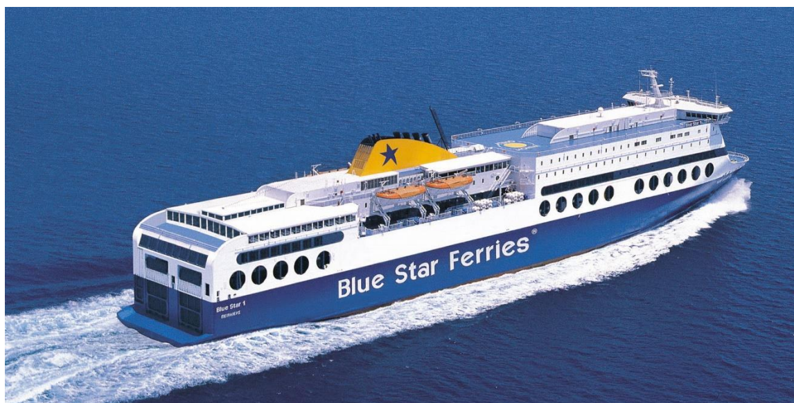
Figure 1-3: Typical stern design and ducktail addition in ro-pax ship Blue Star 1. Source: www.attica-group.com .
