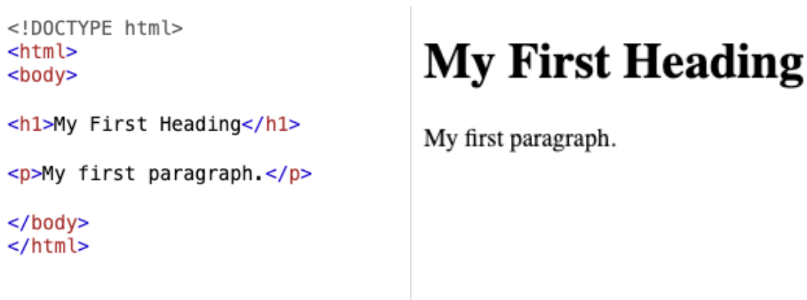
Figure 7: HTML Example of A Simple page (Result in a web browser on the right)
