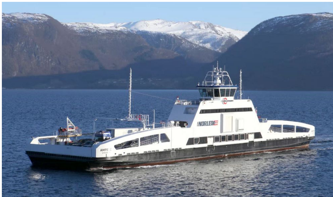
Figure 1: MV Ampere - First all-electric ferry (2015) (1)
