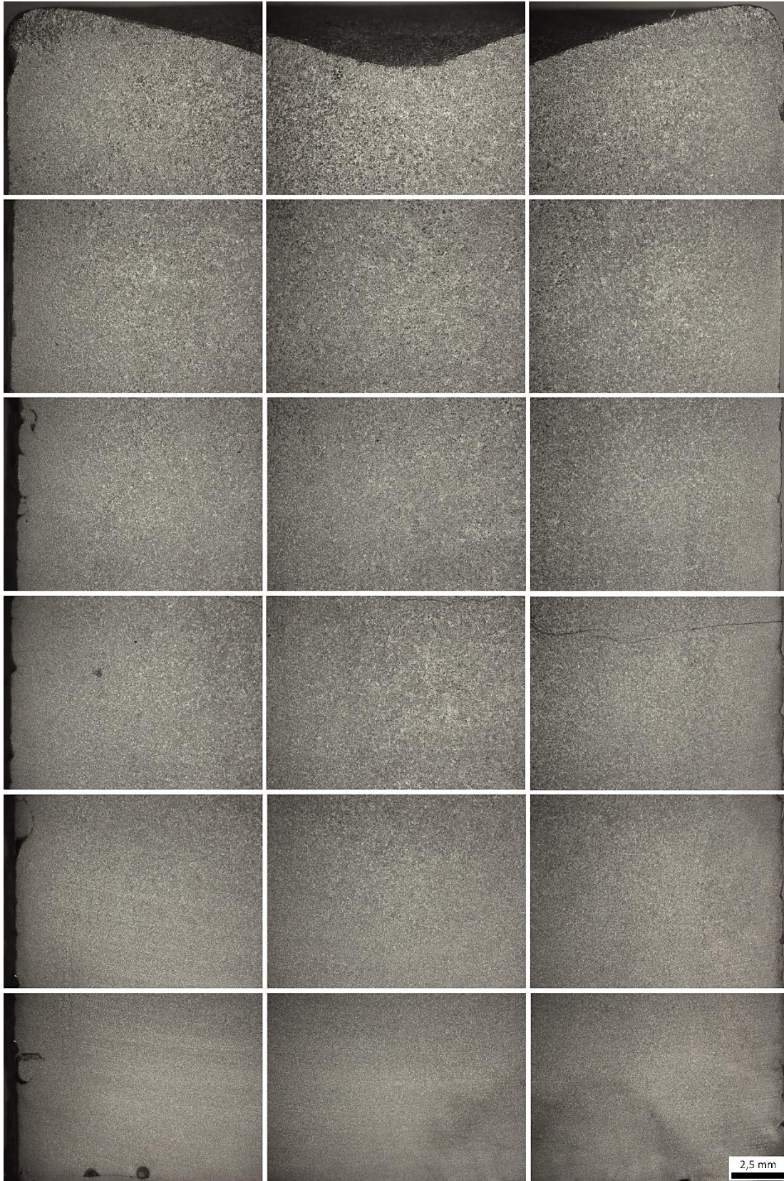
Figure 1. Surface of sample A2 after macroetching with Δ4 etchant (concentrated HNO 3 ).
