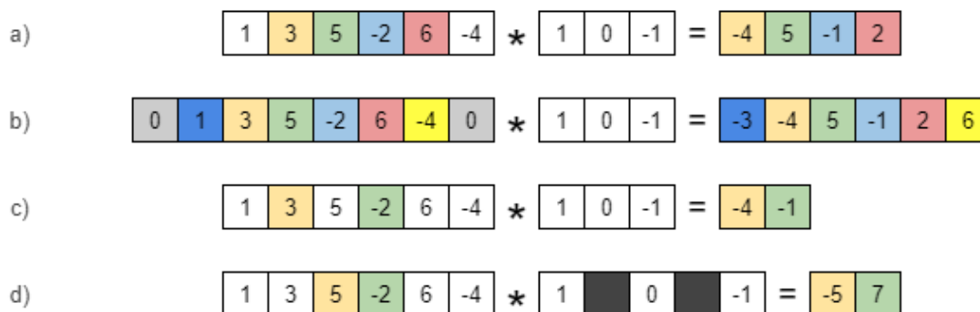
Figure 3.2.3: Plots of 1D convolutions with a kernel of size 3 and various configurations. a) Simple convolution with 1 stride and dilation. b) Convolution when zero-padding is used. Note that the output map is the same size as the input one, with the two edge elements containing possibly false information. c) Convolution with stride of two. d) Dilated convolution with a factor of 2.
