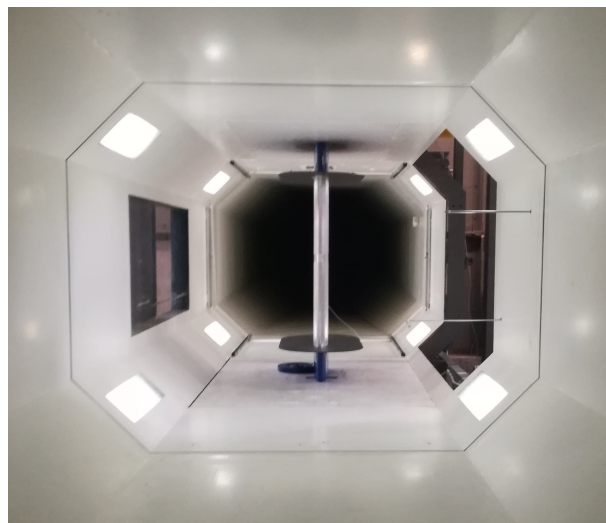
Figure 2.1: The wing model placed inside the test section
