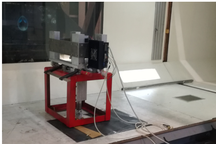
Figure A.3: Photo of the calibration procedure of angular sensor
