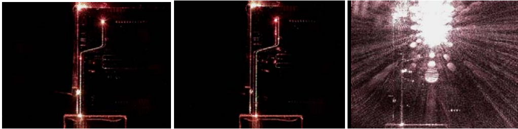
Figure 49: Top view of the grating output for both sides of the grating (left). The right picture shows it for 850 which is saturated due to the 90 degrees output of the chip directly into the camera.
