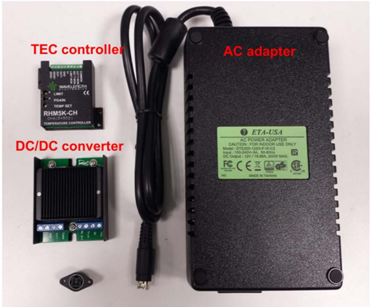
Figure 99: Power supply hardware used in the biophotonic system.
