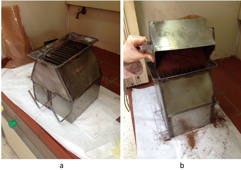
Figure 18. Riffle splitter used to homogenize BR sample
