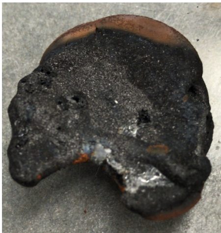
Figure 42. Tablet after 180 seconds irradiation time at 0.6 kW, C/BR 0.180 and 1 l/min nitrogen flow
