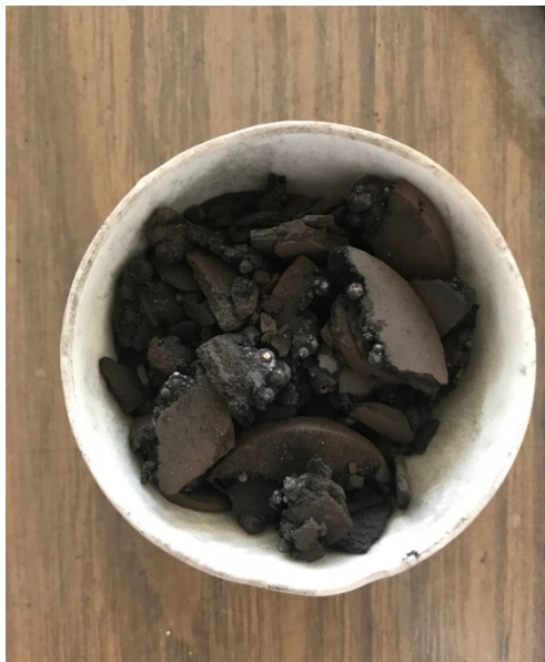
Figure 52. Cinder after 300 seconds, irradiation time at 0.6 kW, C/BR 0.225 and 1 l/min nitrogen flow
