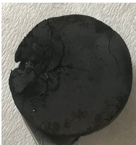
Figure 43. Tablet after 300 seconds irradiation time at 0.6 kW, C/BR 0.180 and 1 l/min nitrogen flow
