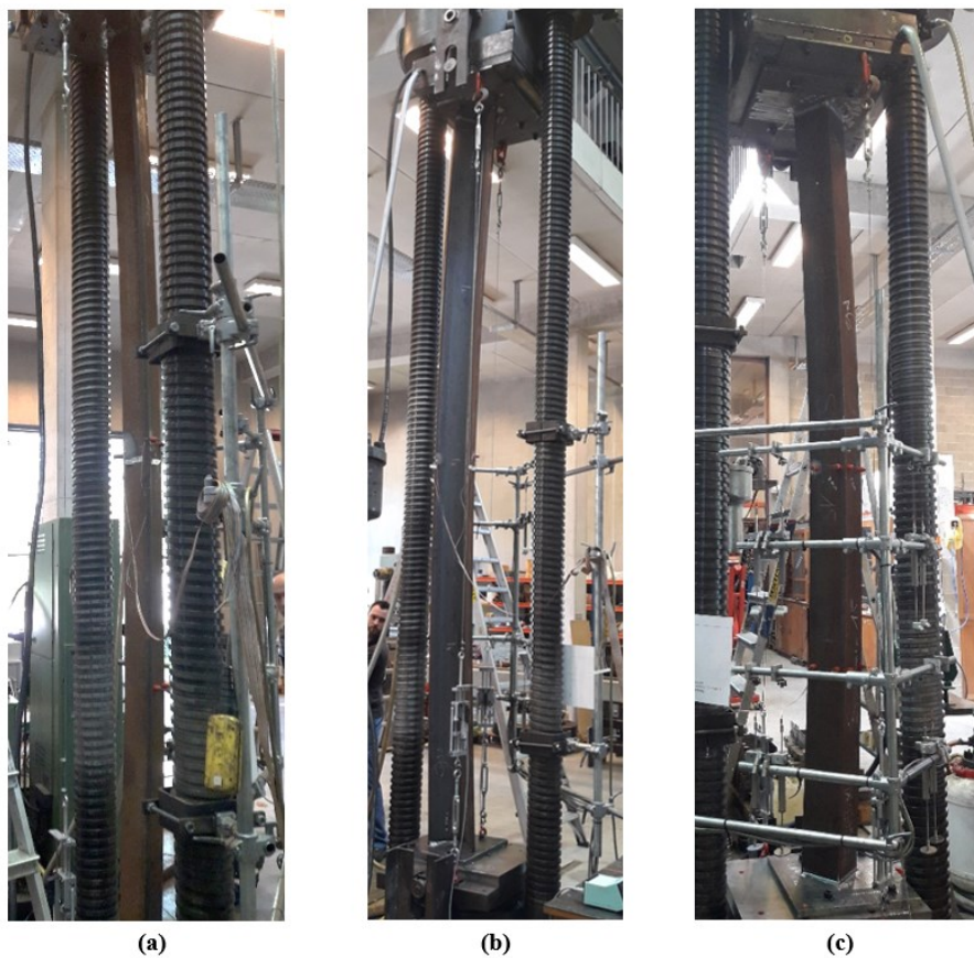
Figure 6.15: Final deformed shape of (a) Sp15 with a pure flexural buckling mode, (b) Sp26 with a flexural-torsional failure buckling mode and (c) Sp14 with a mixed mode between flexural and flexural torsional buckling
