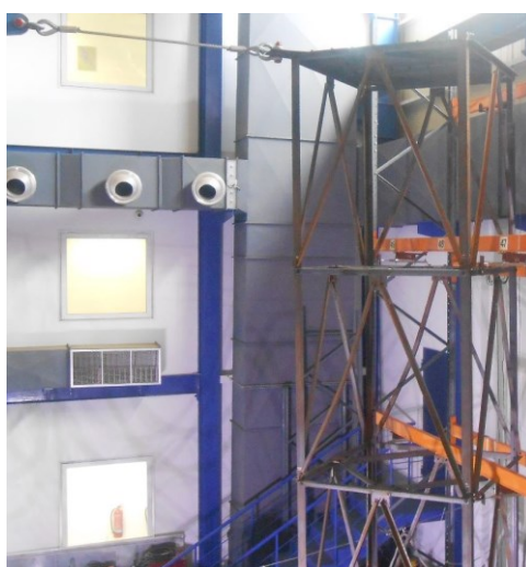
Figure 13.2: Tested tower with diagonal loading [51]
