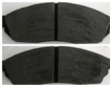
Figure 6 Friction composite by waste tyre rubber particles. (14)
