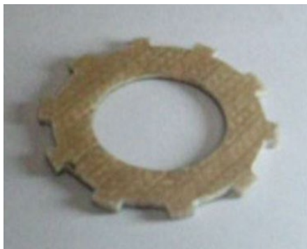
Figure 5 Banana and kenaf woven hybrid composite, (13)
