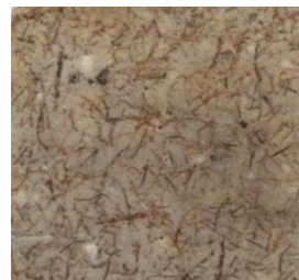
Figure 8 Coconut based composite specimen. (16)
