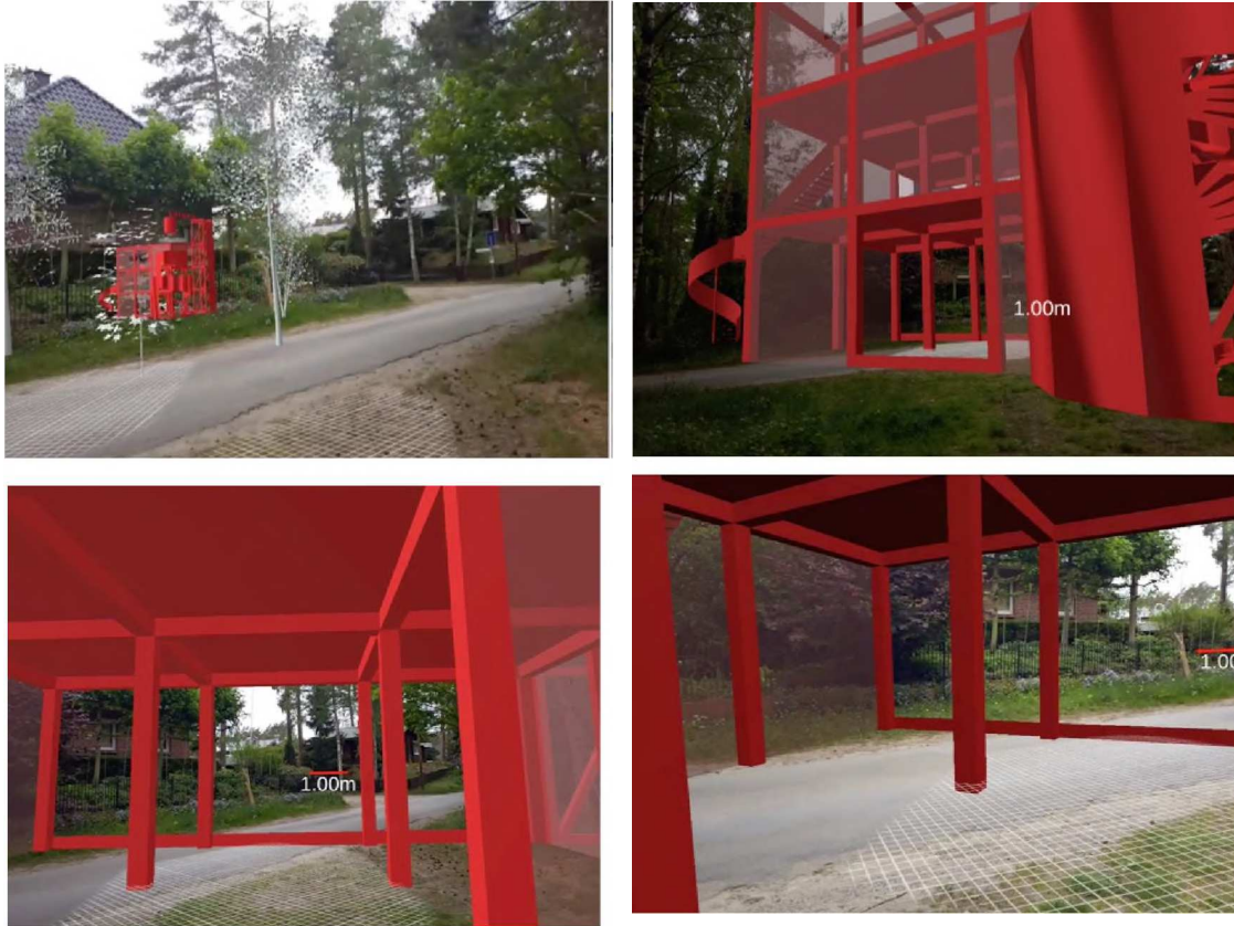
Figure 4. Placing the 3D model of the Folie N5 in another location and exploring the Ground Floor. The limitation with ARtect is that we can explore only the ground floor for now. Further research is needed so the participant can project layers of more floors.
