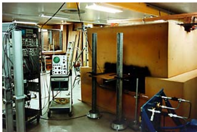
Σχήμα 1.2.8 Stick-slip fault rupture modeling apparatus of two large foam- rubber blocks
