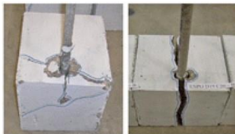
Shape 2.15: Concrete splitting failure
