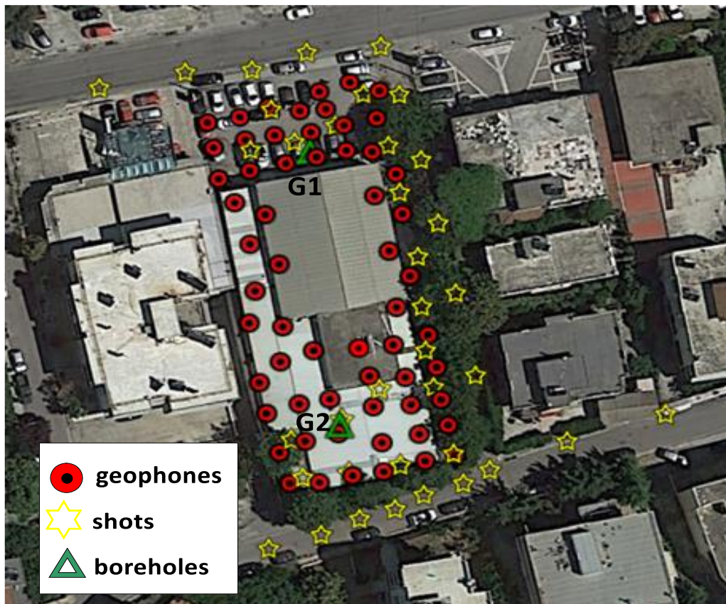
Figure 2. Configuration of the field measurement, red circles represent the approximate location of receivers and yellow stars the location of the seismic sources. The exact position of the two boreholes are represented with the green triangle
