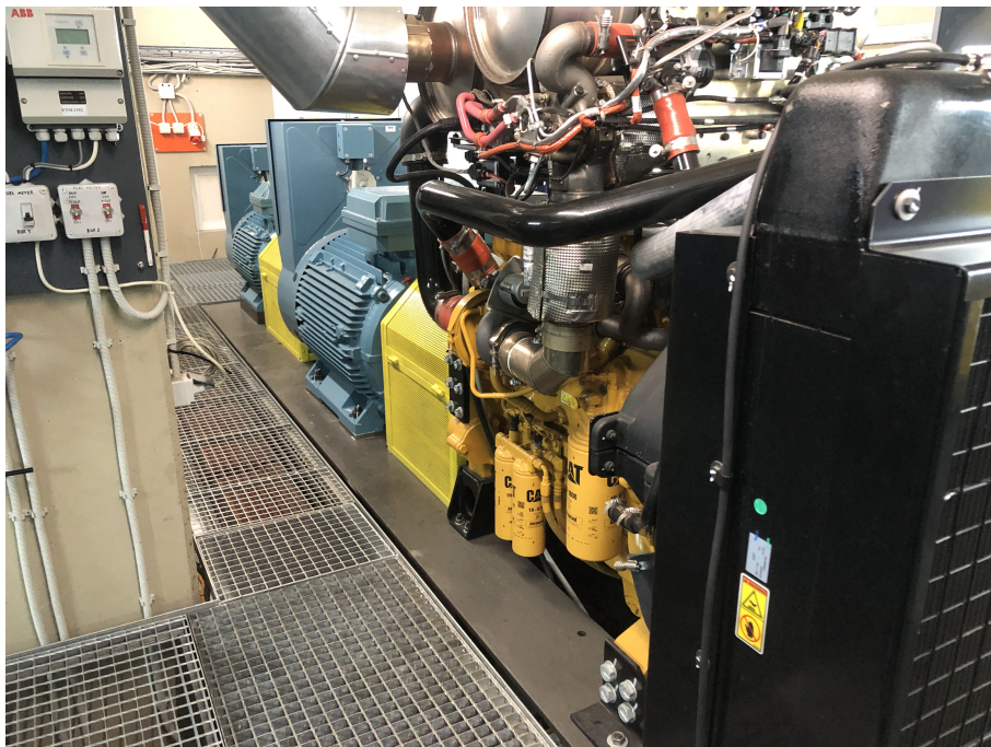
Figure 4.2: Experimental facility in LME showing the first sampling position (near the T/C)
