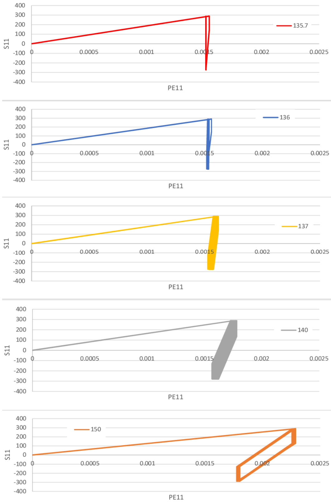
Figure 4.2.6: Stress- Plastic strain diagrams for loads exceeding the shakedown limit.
