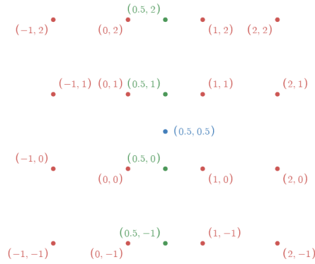
Figure 3.3: Bicubic Convolution Algorithm. The red points form the 4x4 neighbourhood that is to be used to compute the value of the desired pixel. The green dots are the points that will be evaluated when convoluting in the x-dimension. The blue dot is the desired pixel and can be computed by applying convolution in the y-dimension, on the green-dot points.
