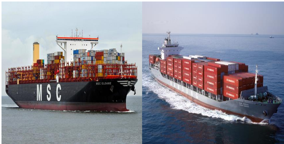
Figure 3.2: Typical ULCV TEUcapacity:19462 L=400m B=58.85m T=15m [46]
