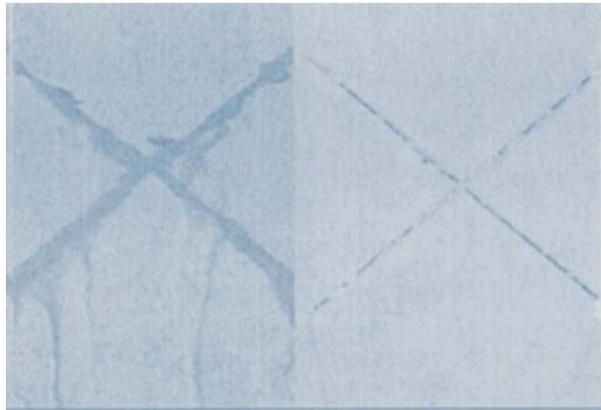
Figure 1.8: Images of coating on steel and aluminum after 240 hours of salt spray [11]
