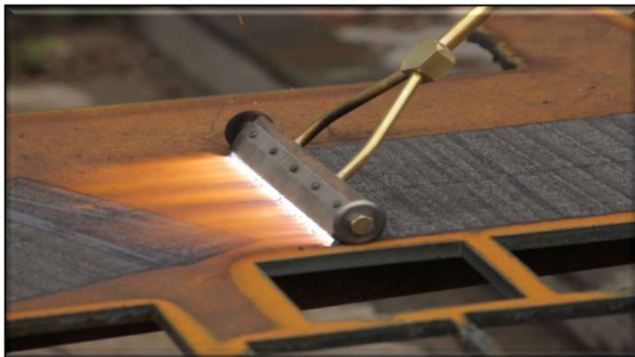
Figure 2.7: Burn marks during the process of flame cleaning [25]
