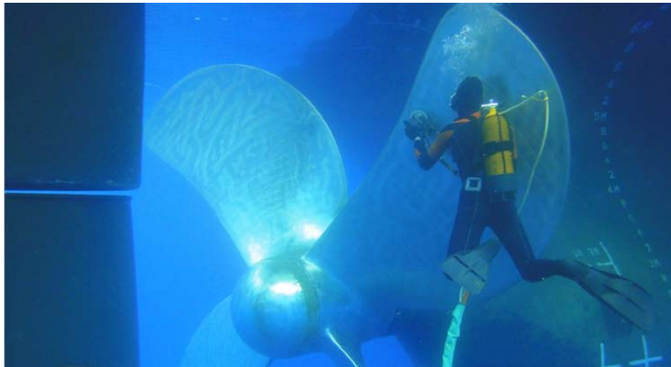
Figure 4.15: Underwater propeller polishing performed by diver [59]
