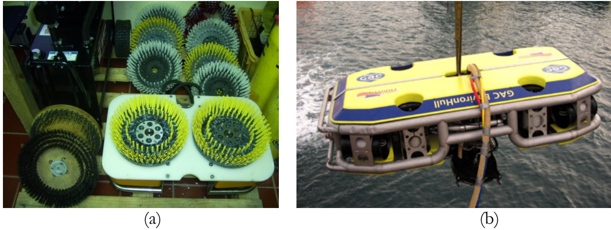
Figure 4.17: (a) Typical example of brushes used for underwater hull cleaning [61] and (b) ROV machine from GAC marine [62]
