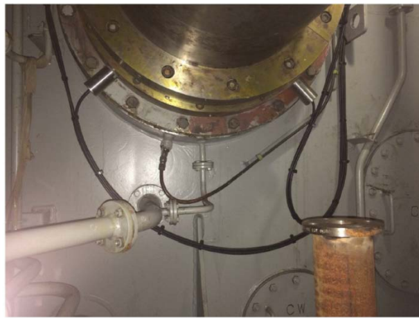
Figure 4.13: Typical forward seal installation of ultrasonic system for propeller protection [57]
