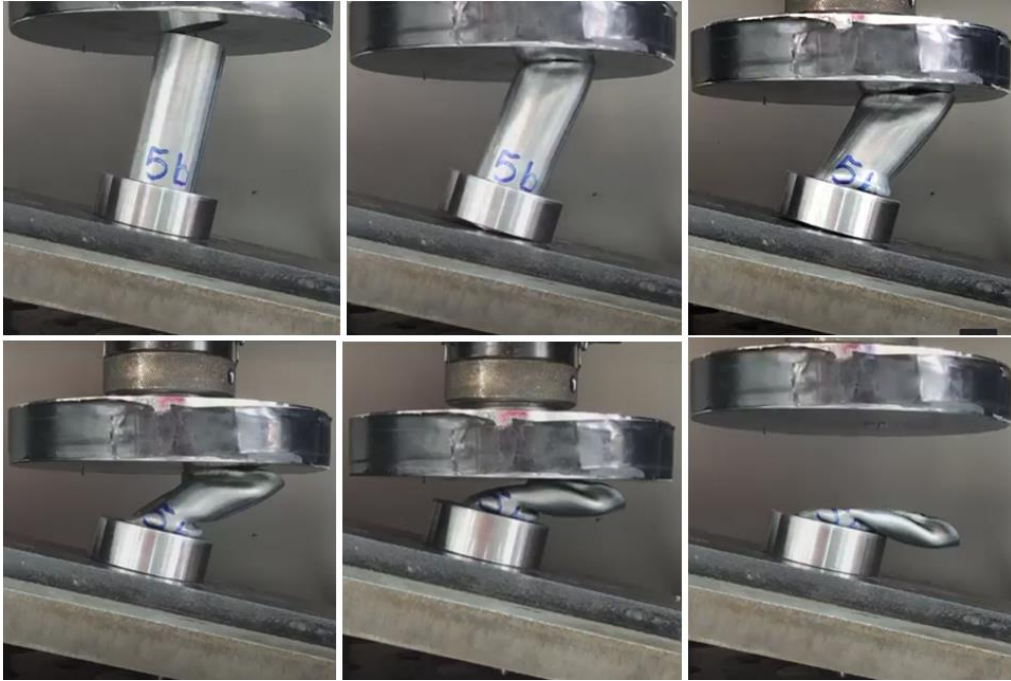
Figure 59 States of specimen 5b oblique collapse
