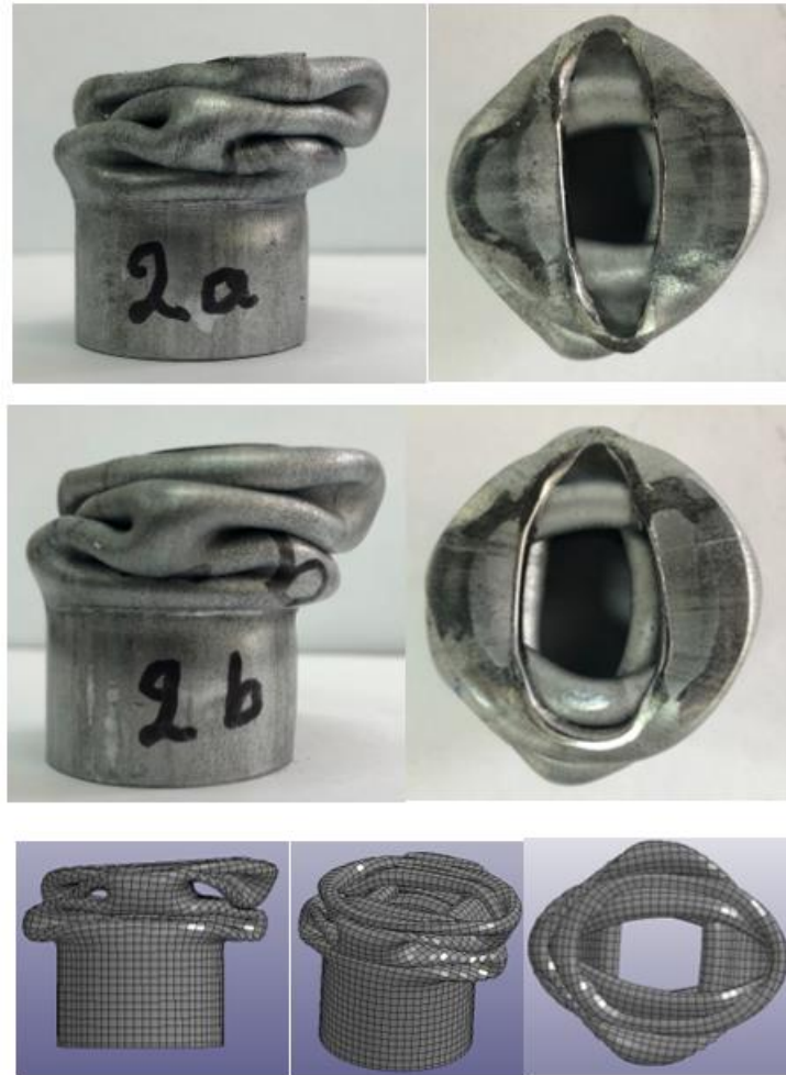
Figure 107 Collapsed structures of specimen 2 (experimental 2a-2b vs. numerical simulation results from top to bottom)
