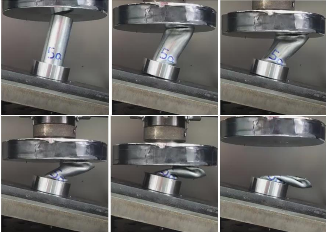
Figure 58 States of specimen 5a oblique collapse
