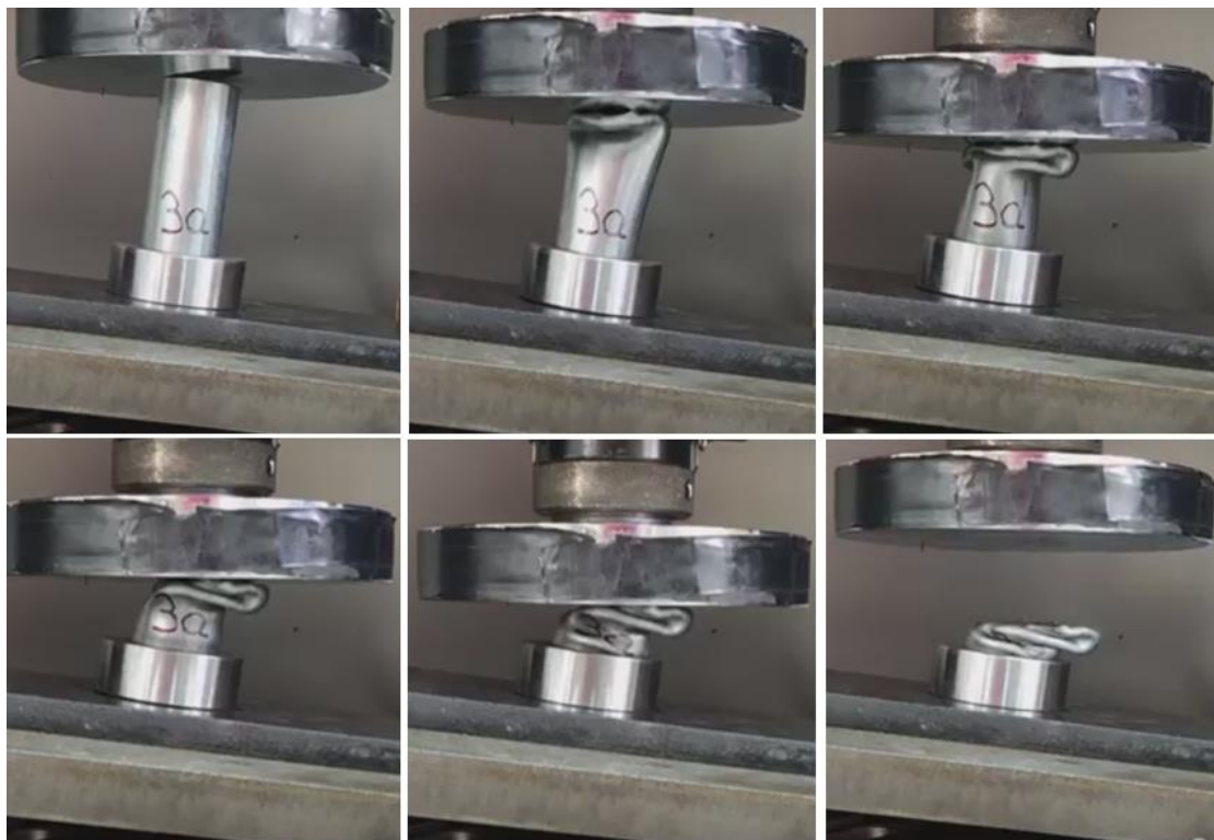
Figure 48 States of specimen 3a oblique collapse
