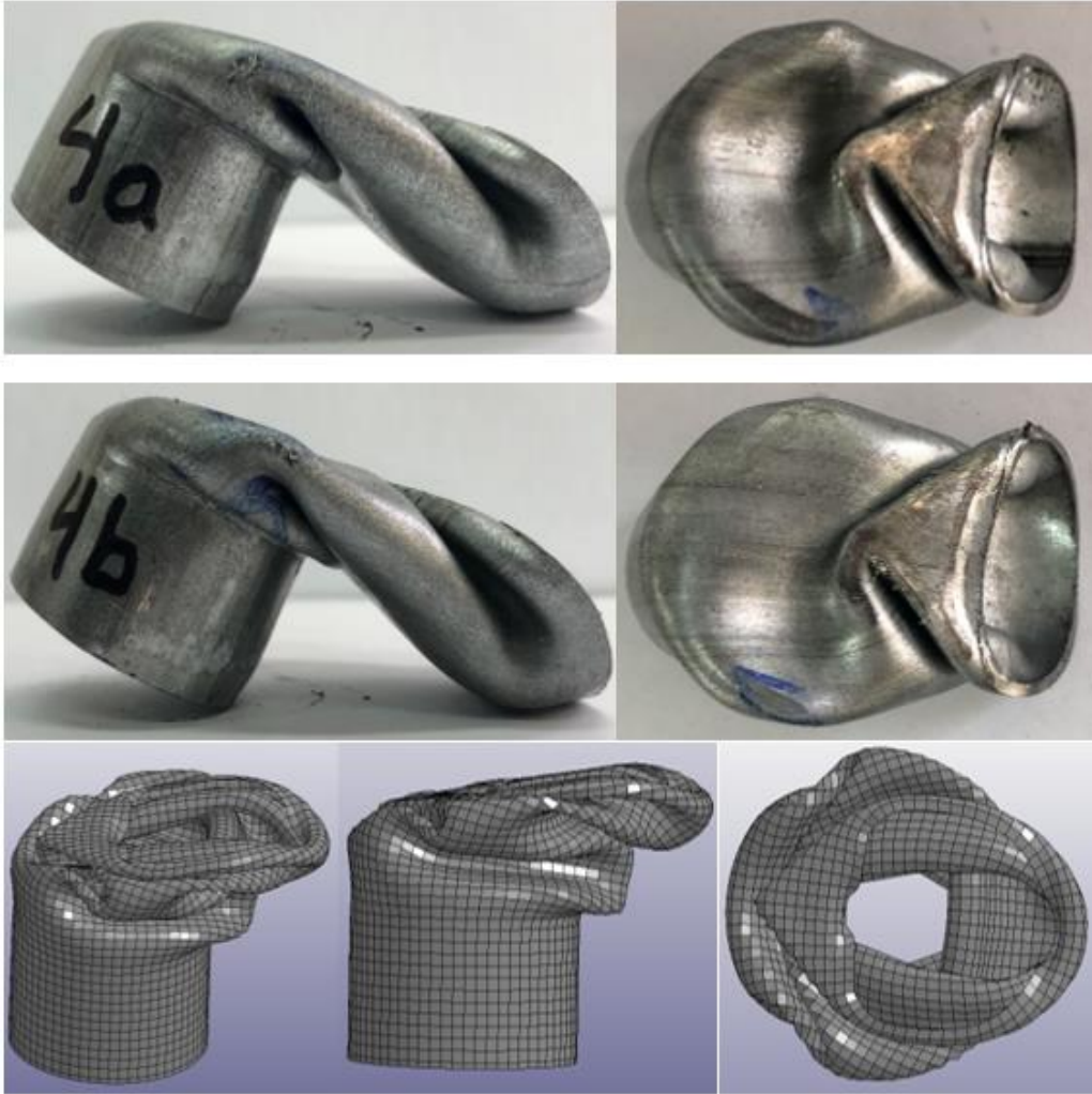
Figure 111 Collapsed structures of specimen 4 (experimental 4a-4b vs. numerical simulation results from top to bottom)
