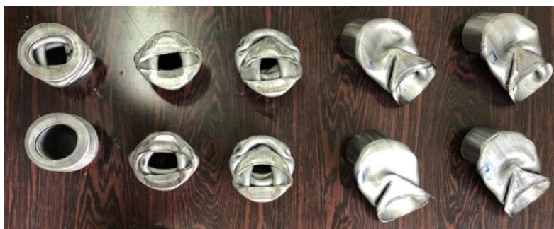
Figure 62 Final views of crushed structures (specimens 1 / 2 / 3 / 4 / 5 from left to right, a: top specimens, b: bottom specimens)
