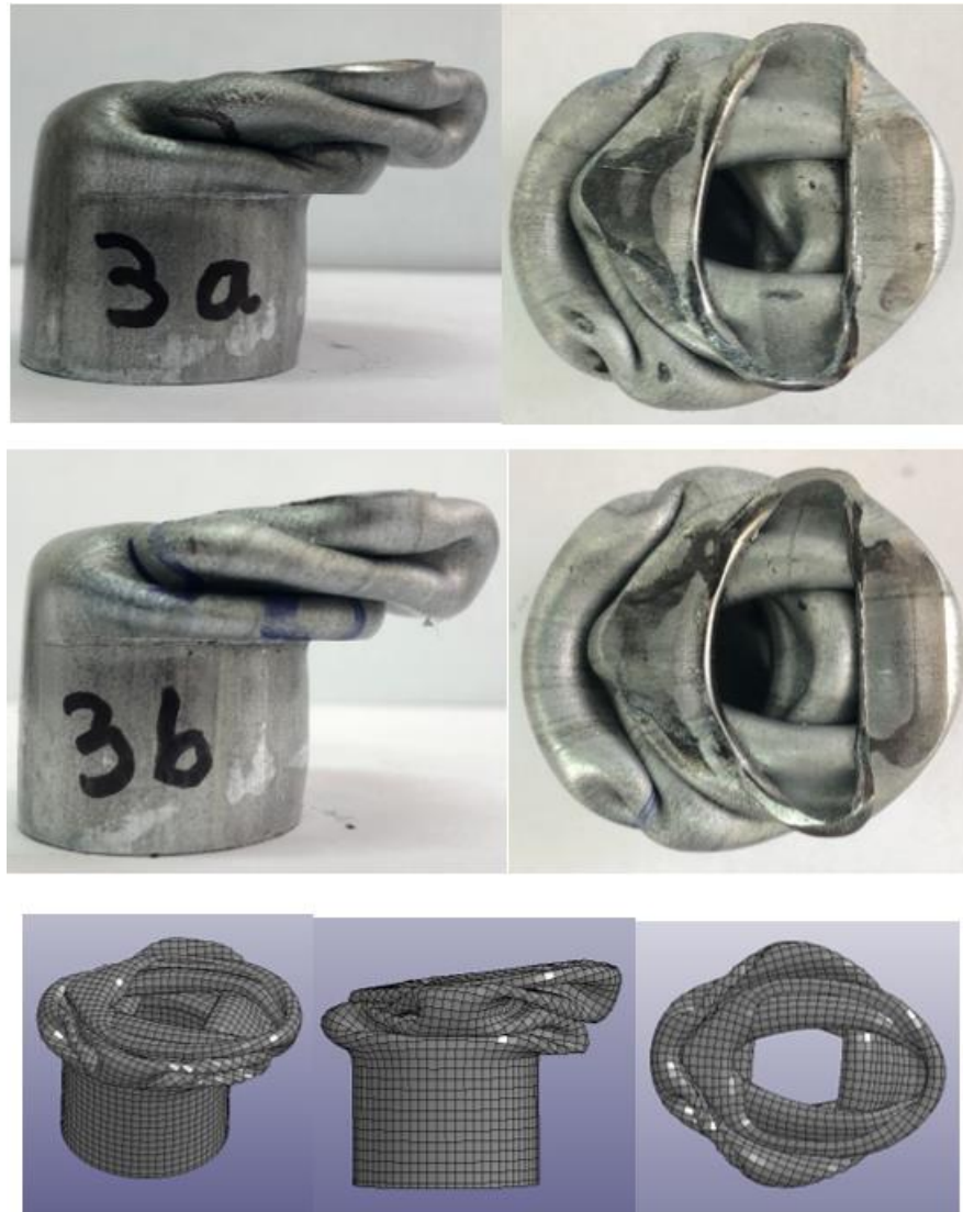
Figure 109 Collapsed structures of specimen 3 (experimental 3a-3b vs. numerical simulation results from top to bottom)
