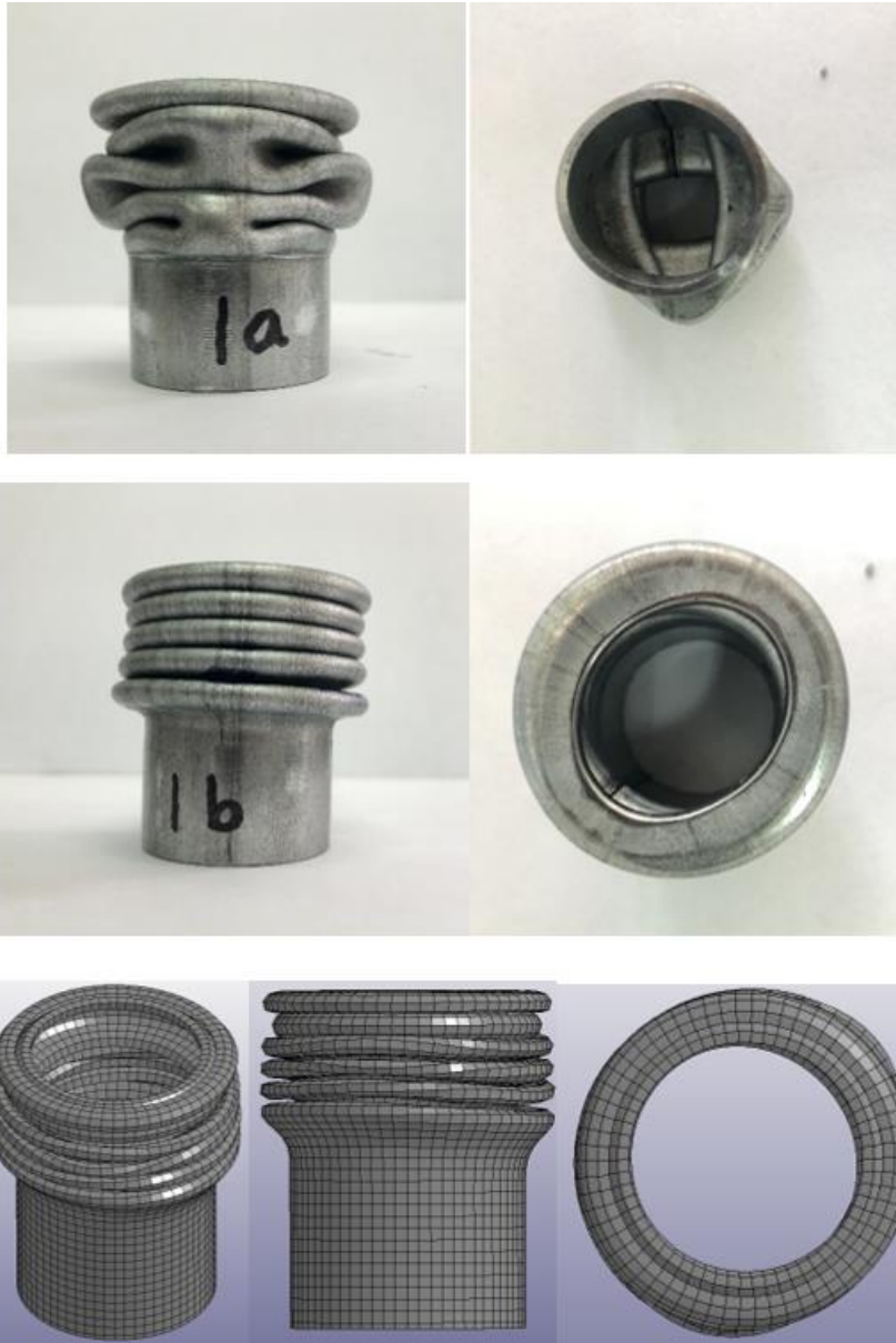
Figure 105 Collapsed structures of specimen 1 (experimental 1a-1b vs. numerical simulation results from top to bottom)
