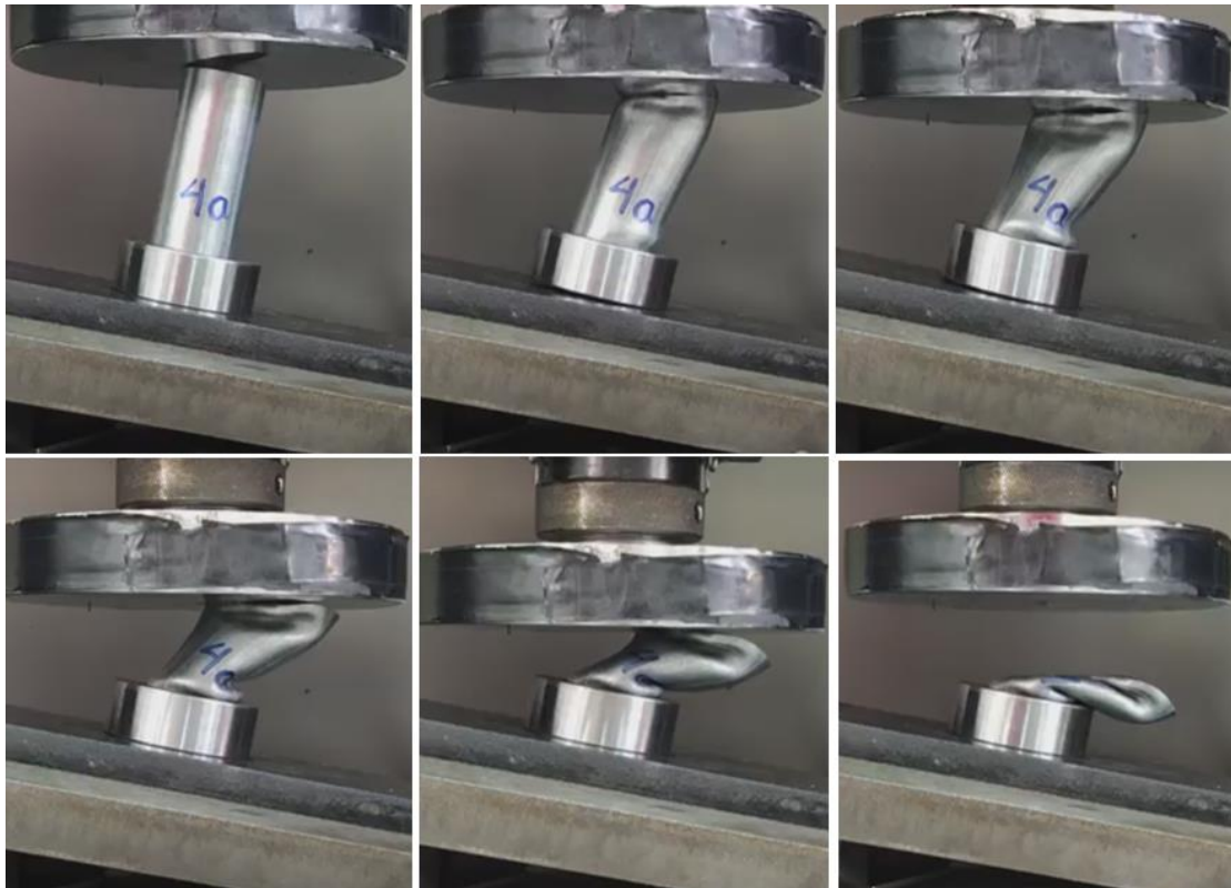
Figure 53 States of specimen 4a oblique collapse
