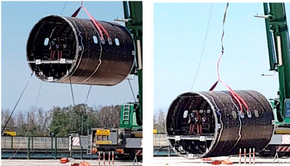
Figure 22 Impact crush test of aircraft's fuselage, [8]
