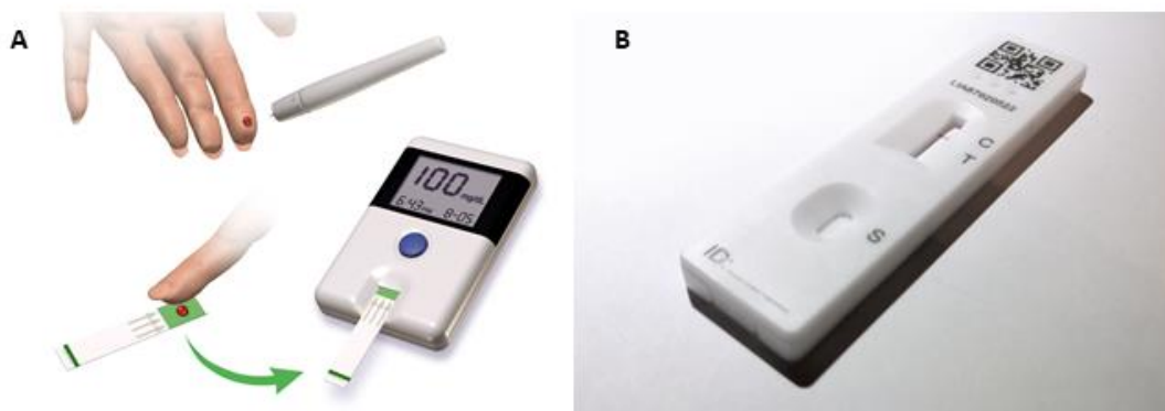
Figure 1.6: Common examples of portable point of care tests: (A) 23 a glucose meter measures blood glucose levels using a drop of blood. (B) 24 A lateral flow test for the detection of an antigen or antibody using immunochromatography, made widely known because of its usage for the detection of SARS-CoV-2 antigen.
