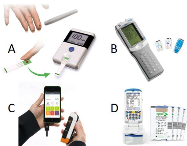
Figure 2.6: Electrochemical biosensing systems: (A) Typical glucose meter (B) i-STAT handheld blood analyzer, Abbott Point of Care inc. (C) Dario's smartphone compatible glucose meter (D) Epoc PoC system by Alere
