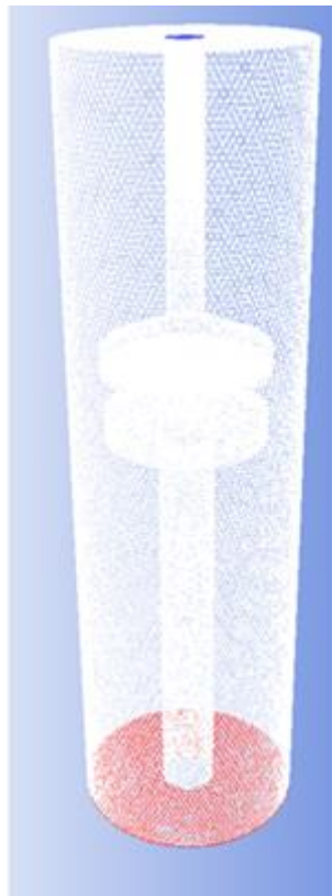
Figure 19: Discretized computational grid of 1232468 FVM cells.
