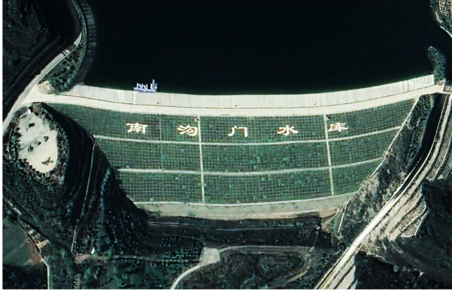
Figure 20. Example of dam with decorative elements and inscription in downstream face – Nangoumen dam (China). Image source: Google Earth capture
