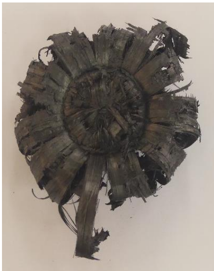
Figure 6.3: Top view of collapsed tube 1a
