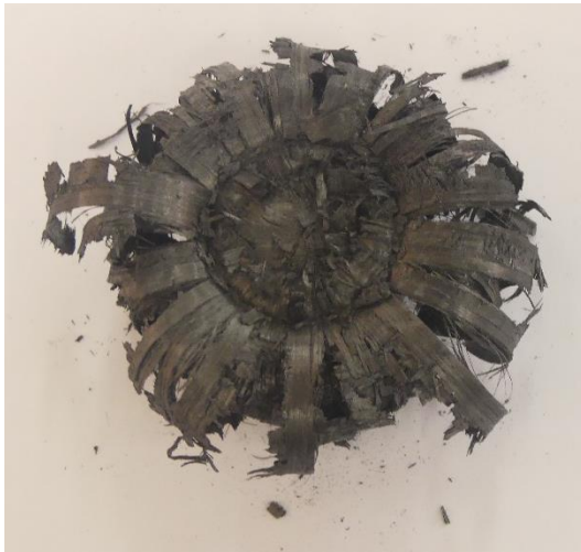
Figure A.9: Top view of collapsed tube 1c
