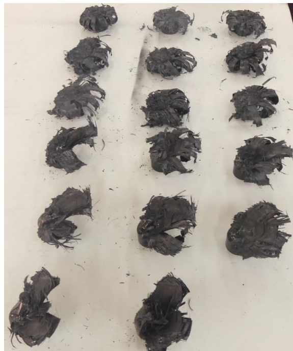
Figure 6.47: All the compressed tubes. Each row corresponds to a different angle. From top to bottom: 0^\circ , 3^\circ , 7^\circ , 12^\circ , 17^\circ and 22^\circ .
