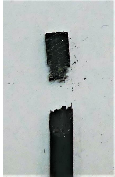
Figure 5.5: Detail of tension coupon 3
