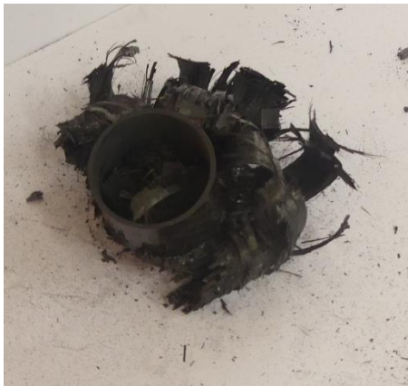
Figure A.57: Bottom view of collapsed tube 4b
