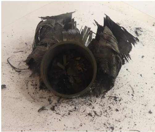
Figure 6.33: Bottom view of collapsed specimen 5c
