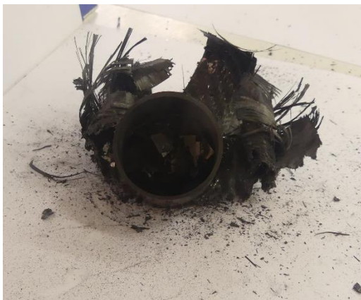
Figure A.65: Bottom view of collapsed tube 5a
