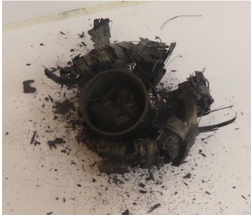
Figure A.41: Bottom view of collapsed tube 3c
