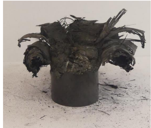
Figure A.56: Left view of collapsed tube 4b
