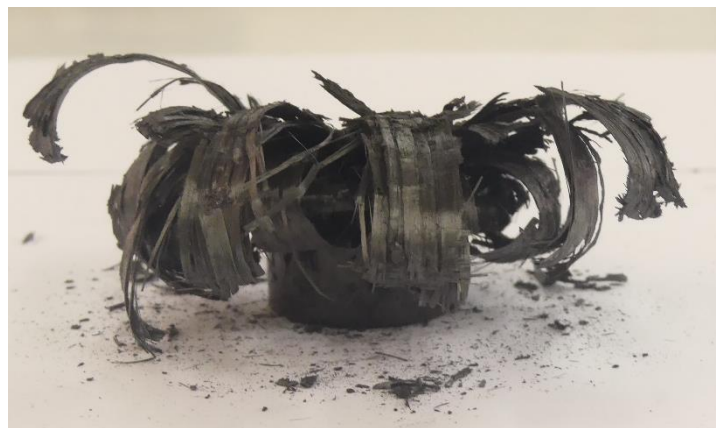
Figure A.34: Right view of collapsed tube 3a
