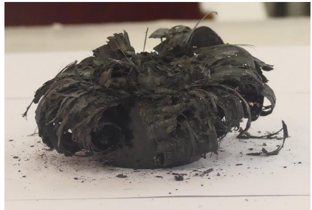
Figure A.24: Left view of collapsed tube 2b
