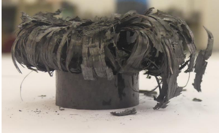
Figure A.2: Front view of collapsed tube 1b
