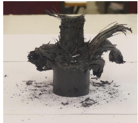
Figure A.48: Left view of collapsed tube 4a
