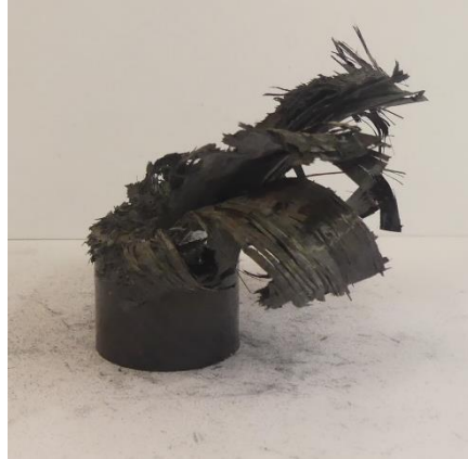
Figure A.46: Front view of collapsed tube 4a
