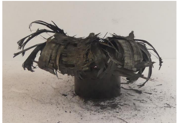
Figure A.58: Right view of collapsed tube 4b
