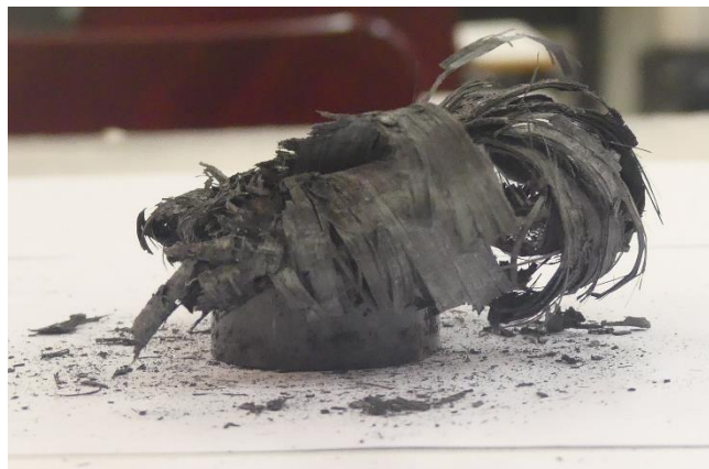
Figure A.38: Front view of collapsed tube 3c
