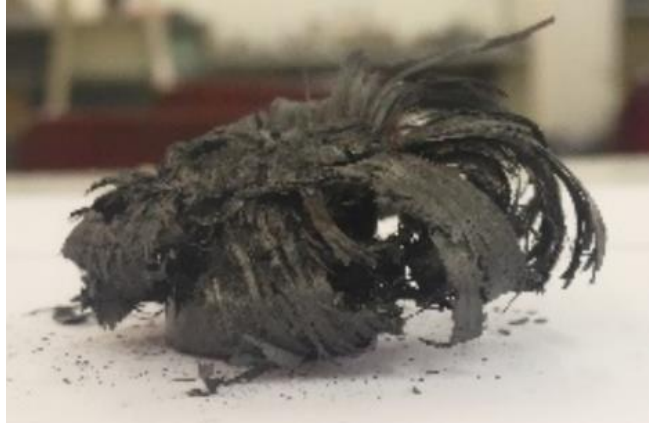
Figure A.14: Front view of collapsed tube 2a
