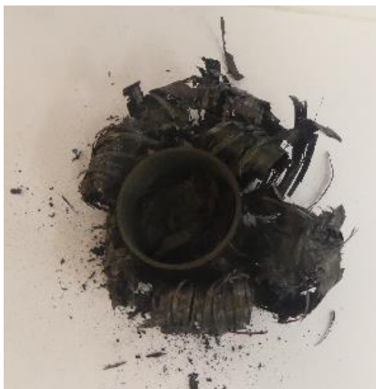
Figure A.17: Bottom view of collapsed tube 2a
