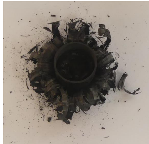
Figure A.10: Bottom view of collapsed tube 1c
