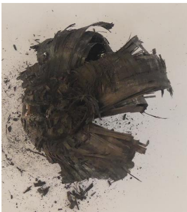
Figure 6.27: Top view of collapsed specimen 4c
