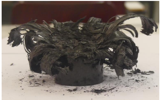
Figure A.32: Left view of collapsed tube 3a
