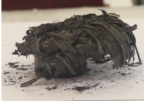
Figure 6.16: Front view of collapsed tube 3b
