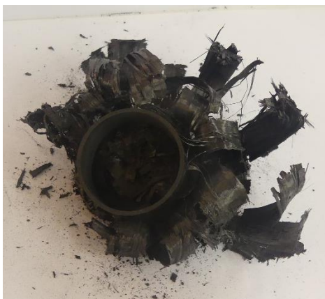
Figure A.33: Bottom view of collapsed tube 3a
