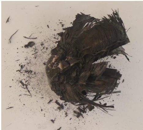
Figure A.63: Top view of collapsed tube 5a
