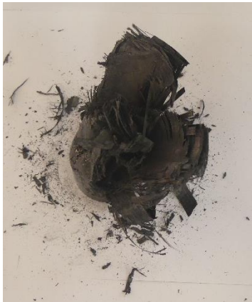
Figure 6.43: Top view of collapsed specimen 6b
