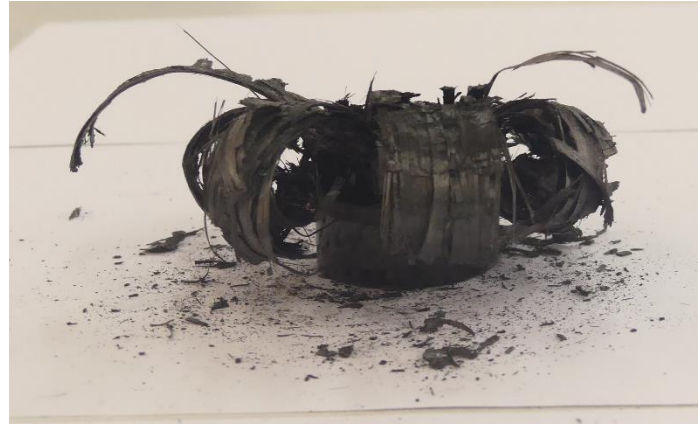
Figure A.42: Right view of collapsed tube 3c
