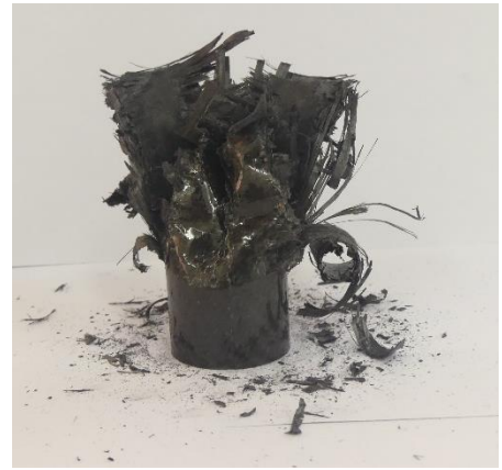
Figure 6.42: Left view of collapsed specimen 6b
