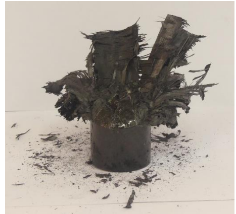
Figure A.64: Left view of collapsed tube 5a
