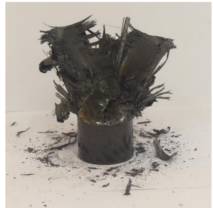
Figure A.80: Left view of collapsed tube 6a
