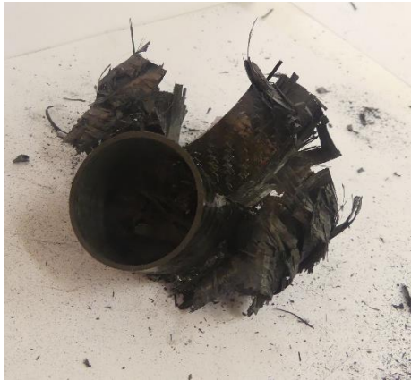
Figure 6.25: Bottom view of collapsed specimen 4c
