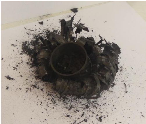
Figure 6.11: Bottom view of collapsed tube 2c
