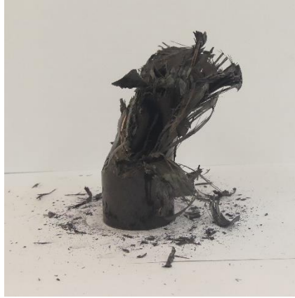
Figure 6.40: Front view of collapsed specimen 6b
