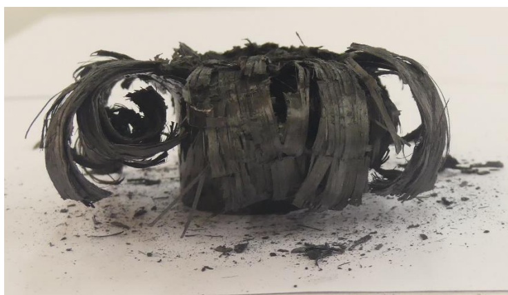
Figure 6.20: Right view of collapsed tube 3b
