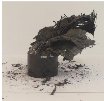
Figure A.70: Front view of collapsed tube 5b
