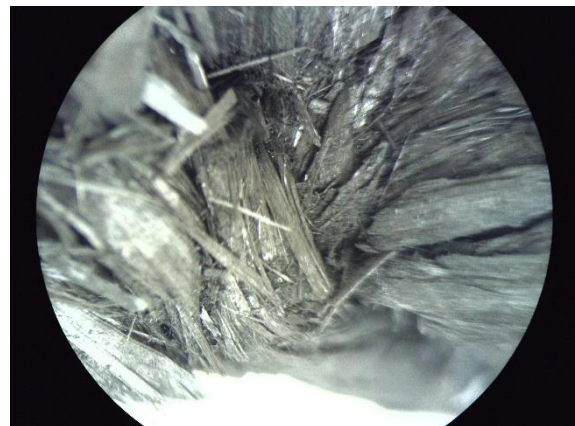
Figure 8.2: 0 deg. loaded specimen. The compression and fragmentation of the inwards bended lamina bundles are apparent.
