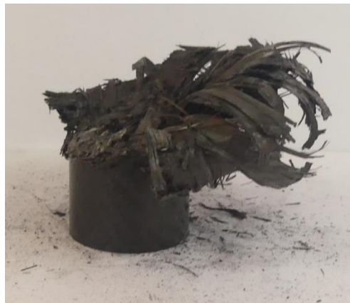
Figure A.54: Front view of collapsed tube 4b
