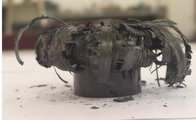
Figure A.8: Front view of collapsed tube 1c
