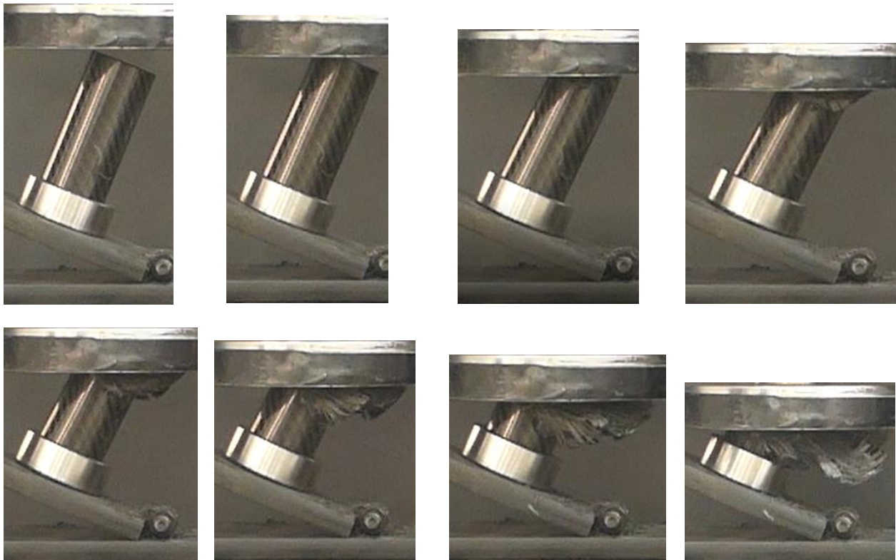
Figures A.77a -h: Stages of collapse of tube 6a
