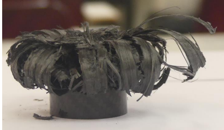
Figure 6.2: Front view of collapsed tube 1a
