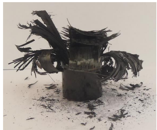
Figure A.66: Right view of collapsed tube 5a
