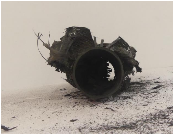
Figure 6.41: Bottom view of collapsed specimen 6b
