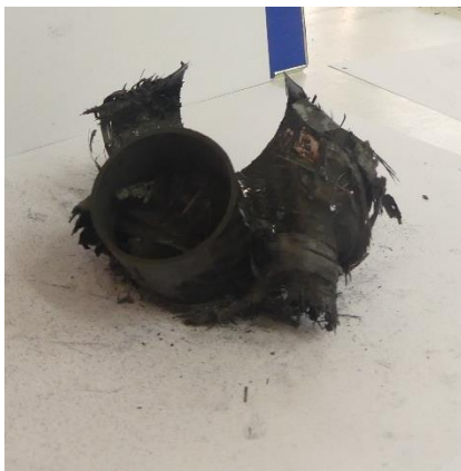
Figure A.49: Bottom view of collapsed tube 4a
