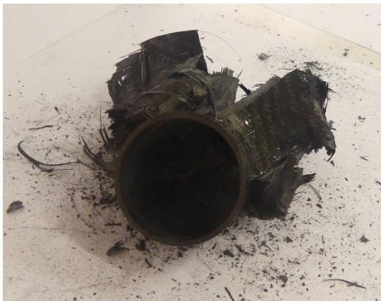
Figure A.81: Bottom view of collapsed tube 6a
