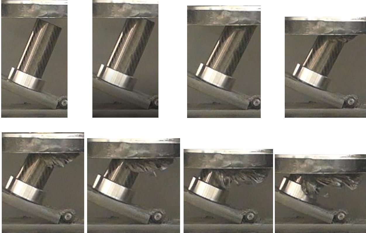
Figures 6.39a – h: Stages of collapse of specimen 6b
