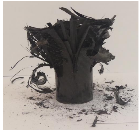
Figure 6.44: Right view of collapsed specimen 6b
