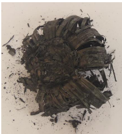
Figure 6.19: Top view of collapsed tube 3b
