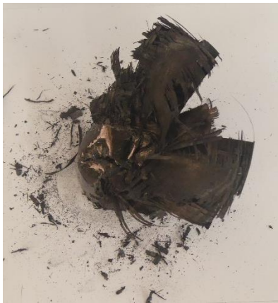
Figure A.79: Top view of collapsed tube 6a
