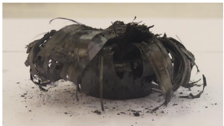
Figure A.26: Right view of collapsed tube 2b
