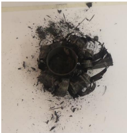
Figure A.25: Bottom view of collapsed tube 2b
