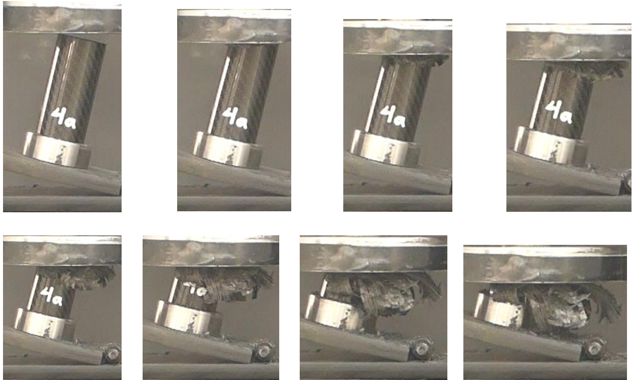
Figures A.45a -h: Stages of collapse of tube 4a
