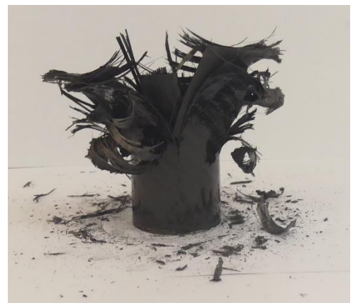
Figure A.82: Right view of collapsed tube 6a
