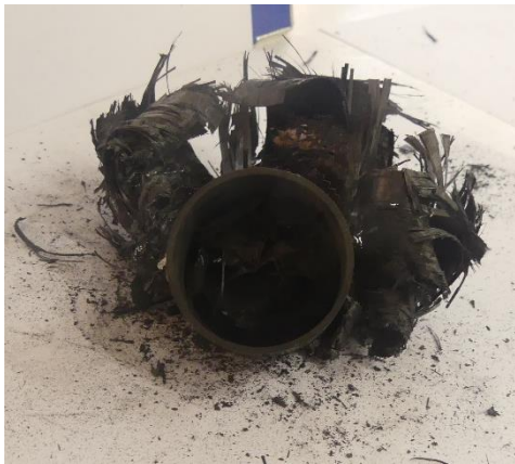
Figure A.73: Bottom view of collapsed tube 5b
