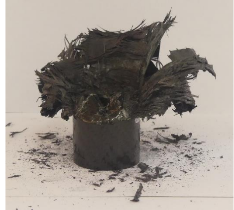
Figure A.72: Left view of collapsed tube 5b
