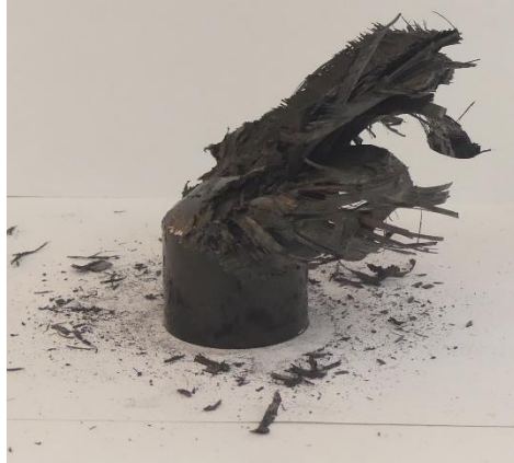
Figure A.62: Front view of collapsed tube 5a
