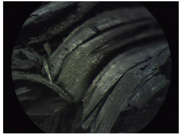
Figure 8.35: 22 deg. loaded specimen. Detail of conflicting inwards bended fronds.
