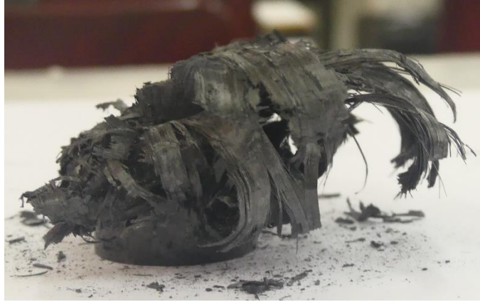
Figure A.30: Front view of collapsed tube 3a
