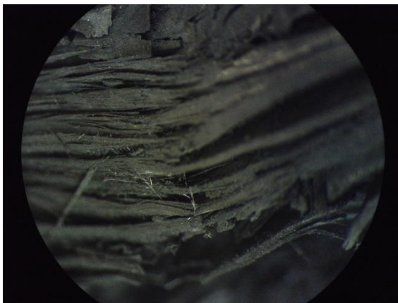
Figure 8.34: 22 deg. loaded specimen. Detail of fracture of the fibers.
