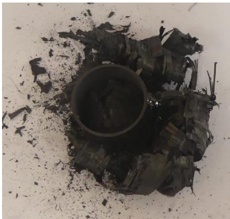
Figure 6.17: Bottom view of collapsed tube 3b
