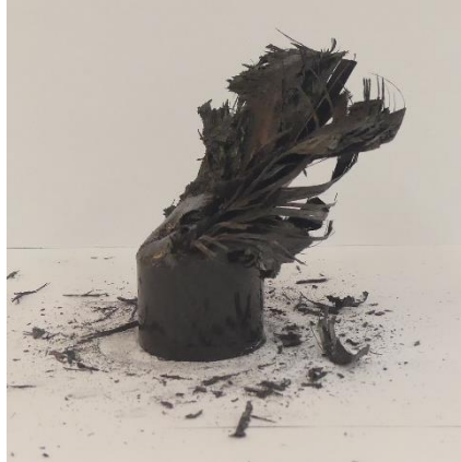
Figure A.78: Front view of collapsed tube 6a
