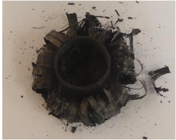
Figure A.4: Bottom view of collapsed tube 1b
