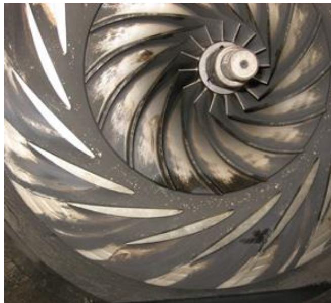
Figure 1-17: Typical T/C fouled compressor 1 .
