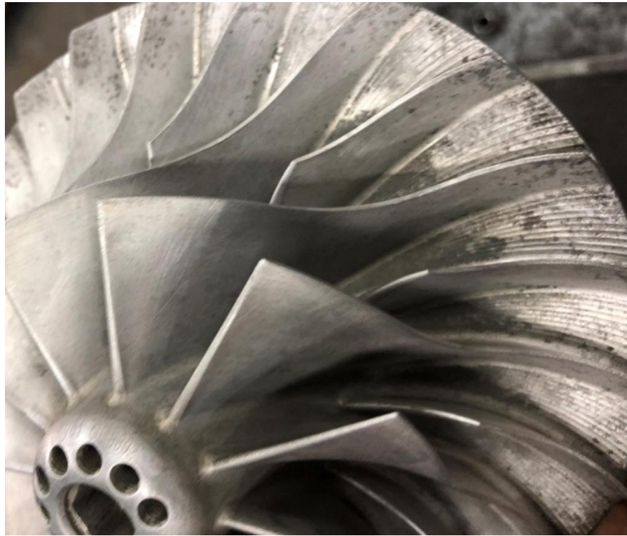
Figure 7-1: Fouled Compressor Impeller. 1
