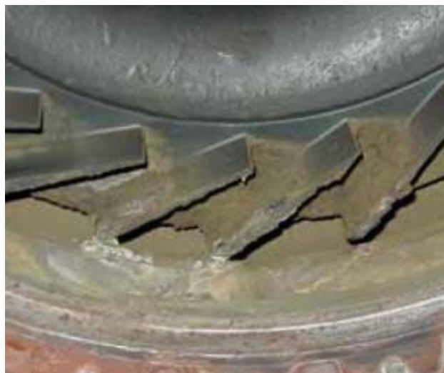
Figure 7-2: Fouled Turbine vaned nozzle 2 .
