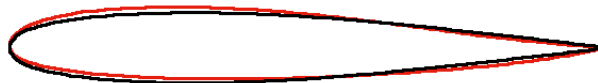
Figure 8.6: NACA0012 airfoil optimization, laminar flow, incompressible fluid: Comparison between the baseline (black) and optimized (red) airfoil after 20 cycles.
