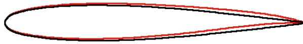
Figure 8.21: Pitching NACA0012 airfoil optimization, inviscid flow, compressible fluid: Comparison between the baseline (black) and optimized (red) airfoil contours.
