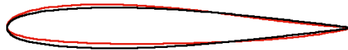
Figure 8.15: NACA0012 airfoil optimization, laminar flow, compressible fluid: Comparison between the baseline (black) and optimized (red) airfoil contours.
