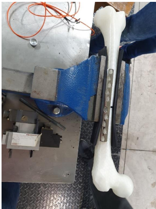
Image 5.6 (left) – Placement of the DCP on the 3D printed femur model
