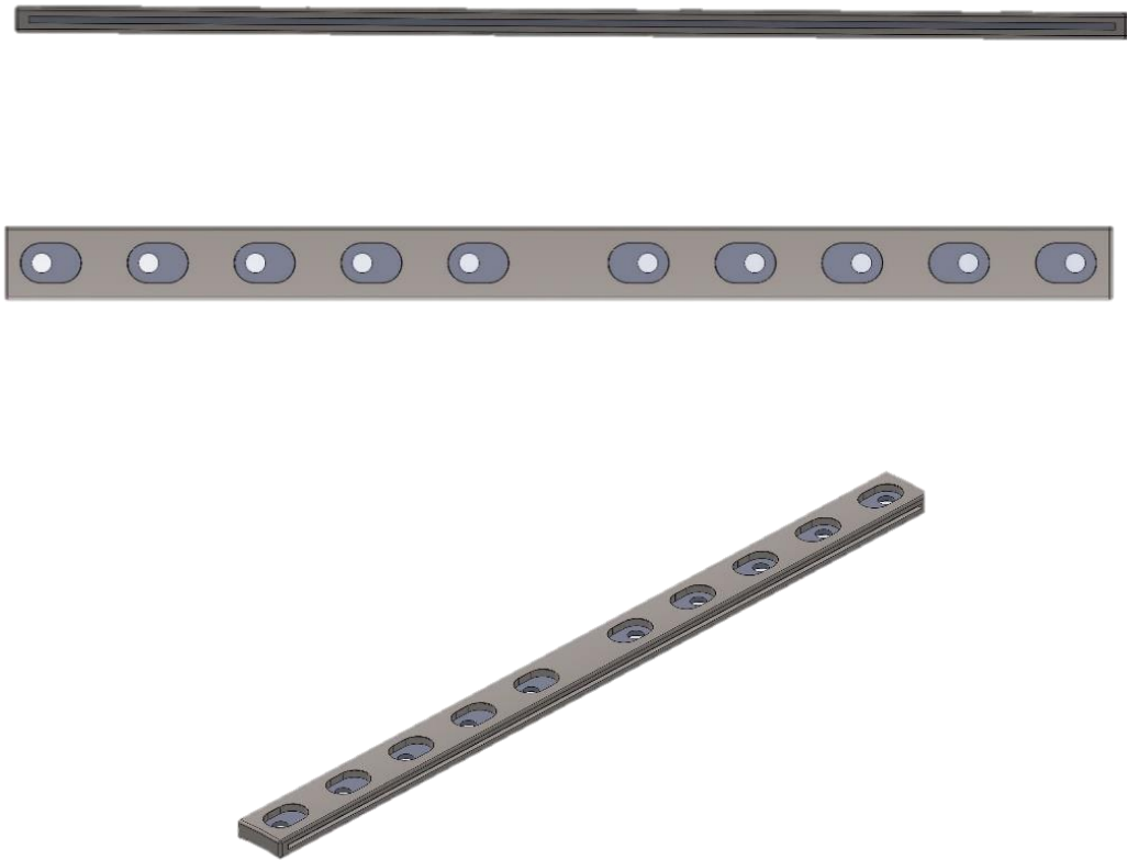
Figure 4.15 – Advanced concept for the screw connector, using a titanium case and a superelastic inner plate
