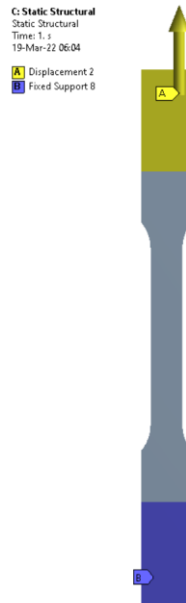
Figure 5.8 - Loading conditions for the tension test specimen model in the ANSYS Static Structural interface
