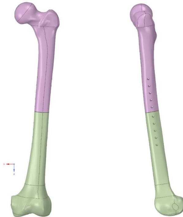
Figure 3.2 - Femur model with holes in the ANSYS Spaceclaim interface
