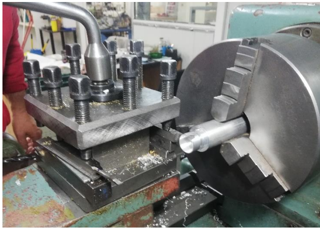
Image 5.8 – Cutting of an aluminum cup from a rod using a lathe machine
