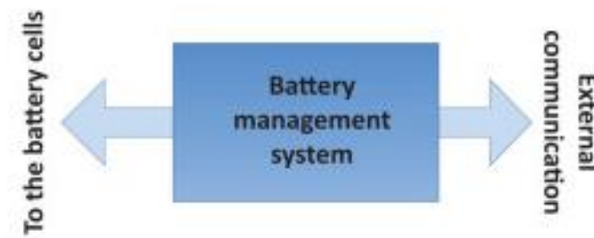
Figure 5.4-2: BMS is the connection between the battery system and the operator
