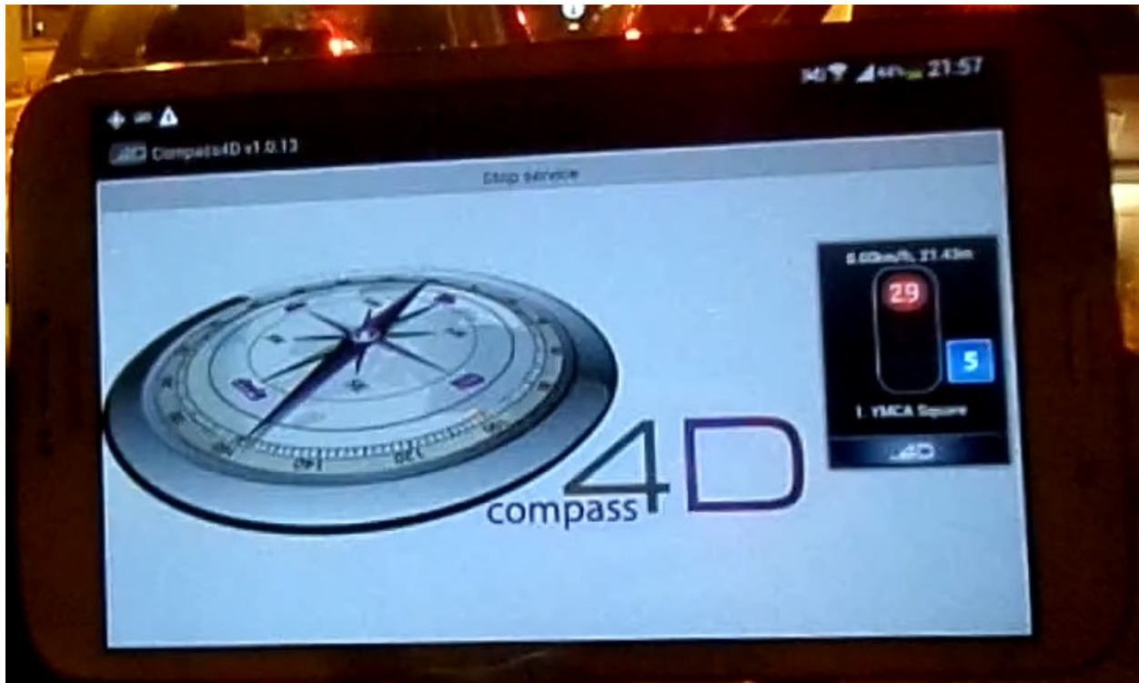
Figure 4.5. OBU (Android Tablet) equipped with 3G/LTE capabilities
