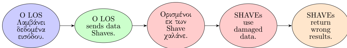
Σχήμα 11: Fault Injection Method: Shaves corrupt their own data.
