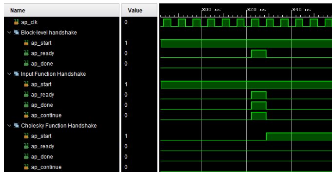
Figure 4.34: Block-level handshake between Input and Cholesky Functions.
