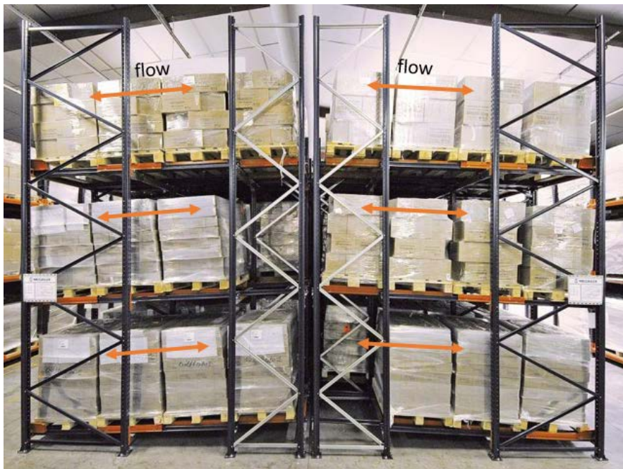
Figure 2.12: Example of a push-back gravity flow racking system (photo courtesy of MECALUX S.A.).
