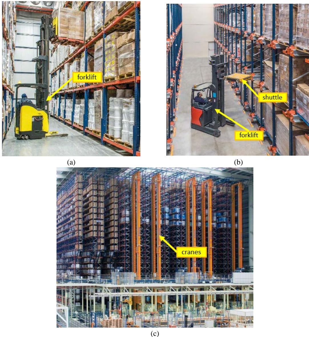
Figure 2.20: Material/goods handling Attribute-Level of the storage system Attribute consists of three Options: (a) manual, (b) semi-automated, and (c) fully-automated (photos courtesy of MECALUX S.A.).
