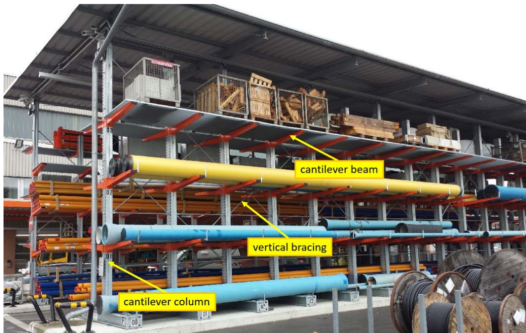
Figure 2.8: Example of a heavy-duty cantilever rack (photo courtesy of Modulblok).
