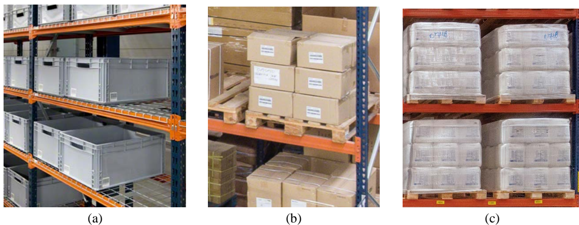
Figure 2.18: The weight of the unit load Attribute-Level of the storage system Attribute consists of three Options: (a) low-, (b) medium- and (c) high-weight (photos courtesy of MECALUX S.A.).
