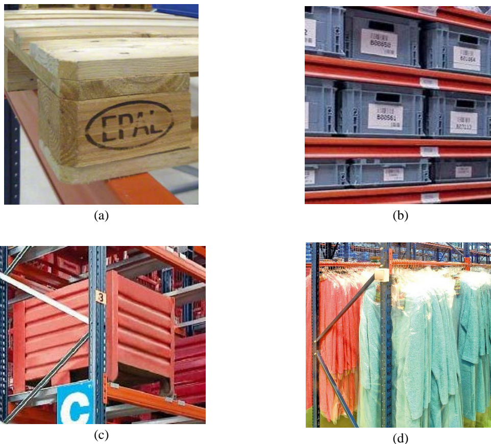
Figure 2.19: The contact surface Attribute-Level of the storage system Attribute consists of four Options: (a) wood+steel, (b) plastic+steel, (c) steel+steel and (d) hanging goods (photos courtesy of MECALUX S.A.).
