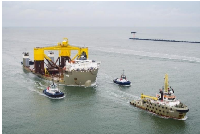
Figure 2-42 Kincardine Offshore Wind Farm semi-submersible foundations being transported to assembly base ( www.projectcargojournal.com )
