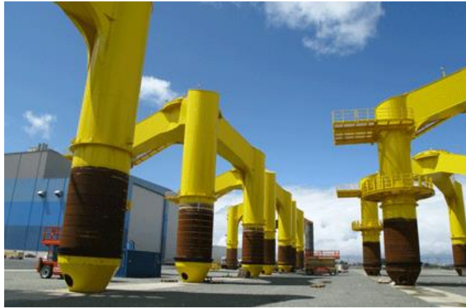
Figure 2-35 Tripiles in Bard's manufacturing base in the German port of Emden ( www.windpowermonthly.com )
