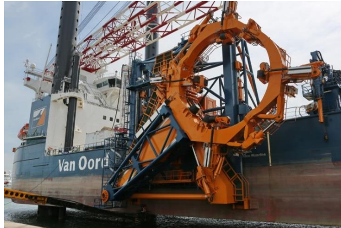
Figure 2-8 Monopile gripper ( www.schuttevaer.nl )
