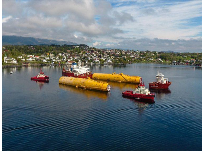
Figure 2-46 Spar buoys being transported from the manufacture base off the project's assembly base ( www.offshorewind.biz )
