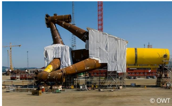
Figure 2-26 Tripod for Alpha Ventus Offshore Wind Farm being welded, transition piece integrated ( www.wikiwand.com )
