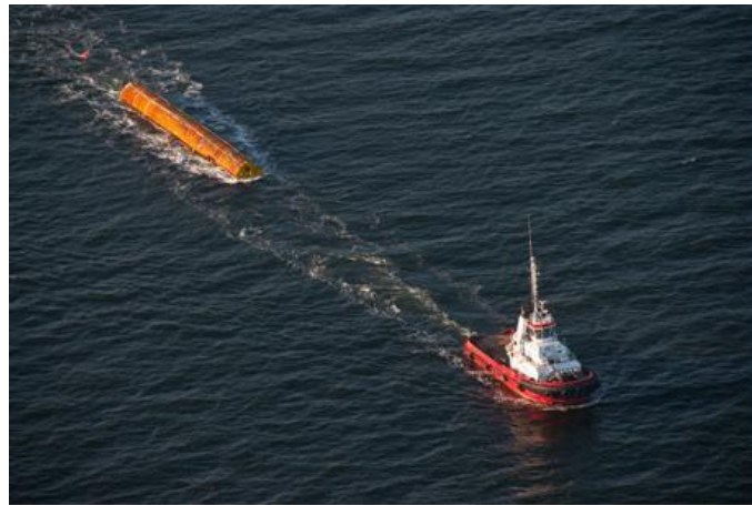
Figure 2-3 Monopile transportation by tug at the Anholt Offshore Wind Farm ( windpoweroffshore.com )
