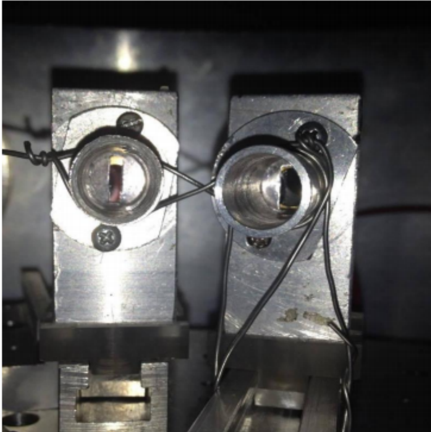
Figure 2.5: Vertical slits placed to constrain the angular uncertainty.
