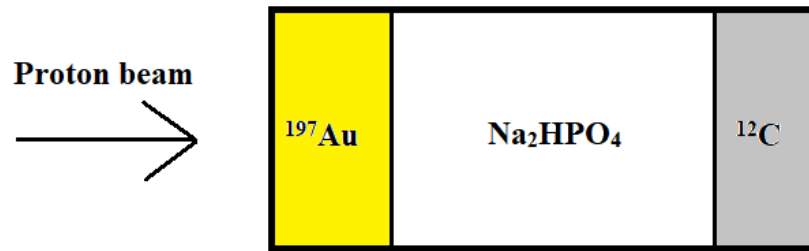
Figure 2.4: A cross section of the three layers of the target.
