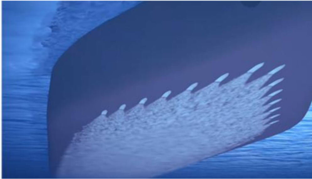
Figure 31: Air lubrication system (20)
