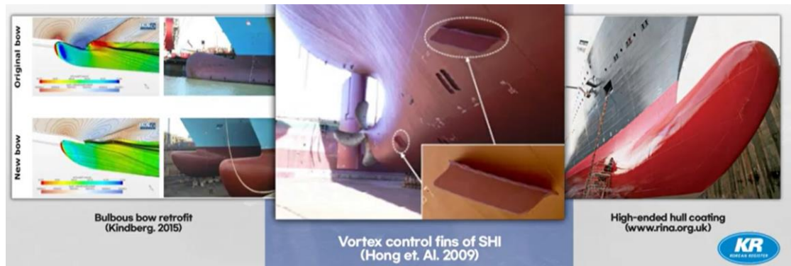
Figure 23: Ship's wave making and friction resistance reduction methods (KR)
