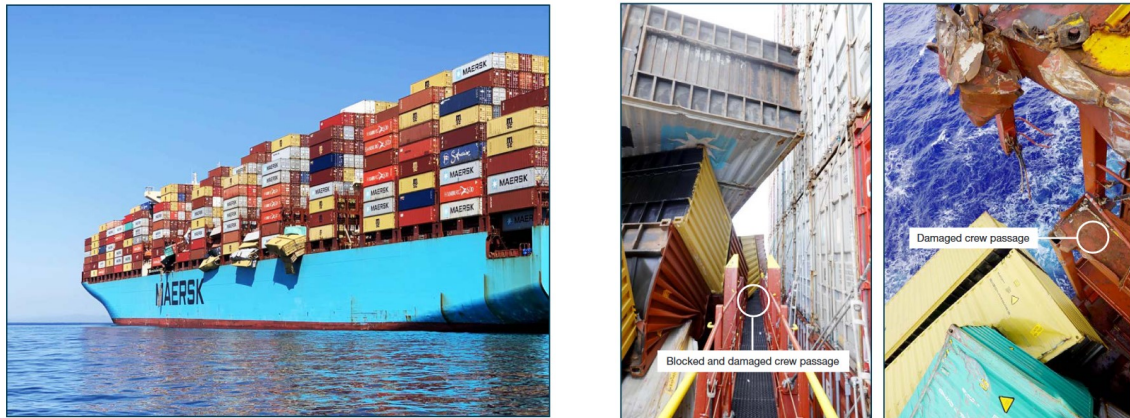
Figure 1.2: Examples of lashing bridge damages and container losses, occurred in MAERSK ESSEN accident [4]
