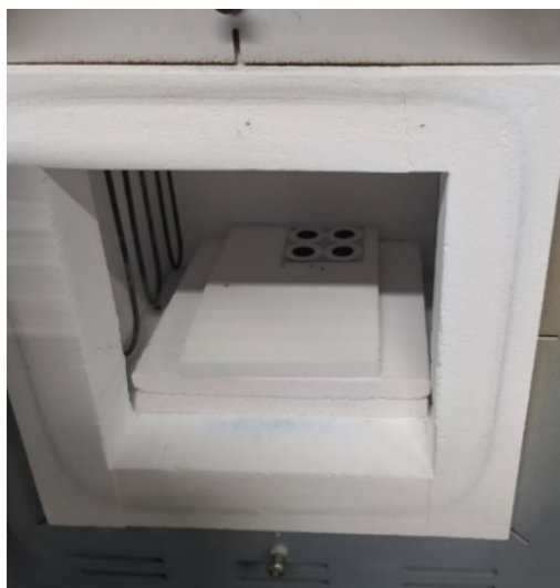
Figure 6.7 Fuel Cell Sintering
