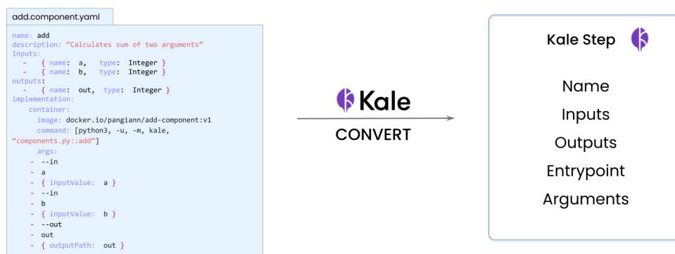
Figure 4.8: The conversion of a YAML file to a Kale step
