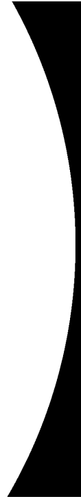
Image 6.19: Example of a lunar Mask. The pixels outside of the limb have a value of 0 and appear black, while the pixels inside of the limb have a value of 255 in 8-bit images and 65535 in 16-bit images (max value) and they appear white.
