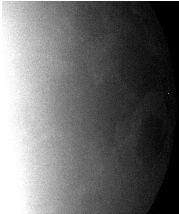
Image 1.1: A validated impact flash, captured by the Krioneri Telescope of the National Observatory of Athens.
