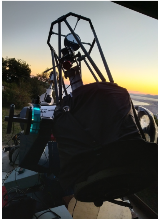
Image 3.6: The 50 cm custom Newtonian telescope used at the Observatoire de la Côte d'Azur.
