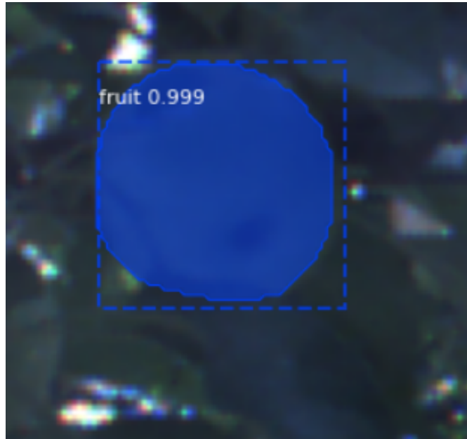
Figure 2.11. This is a detection made using Mask R-CNN. It shows a bonding box(dotted), segmentation mask, class (fruit) and the confidence score(0.999). Object detection model typically outputs the bounding box, confidence score and clas. Confidence value is the confidence of the model on the detection and it ranges between 0 and 1.
