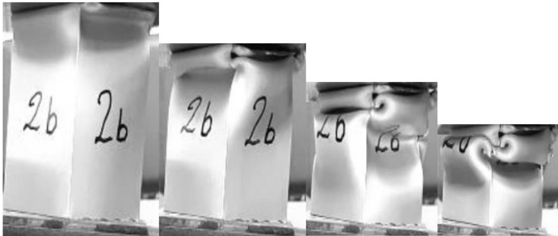
Figure 61 Collapse states of test 2b under contact in corner
