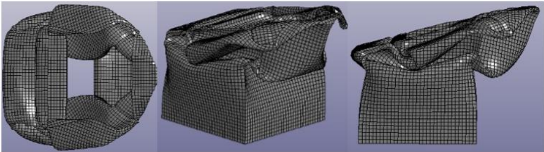
Figure 136 Final views of crushed tube model in simulation case 4 under contact in edge
