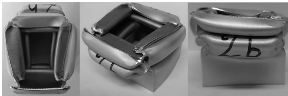
Figure 63 Final views of crushed specimen in test 2b under contact in corner
