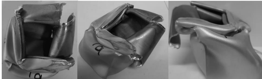
Figure 87 Final views of crushed specimen in test 4b under contact in corner
