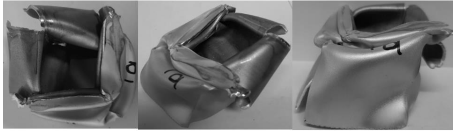
Figure 86 Final views of crushed specimen in test 4a under contact in corner
