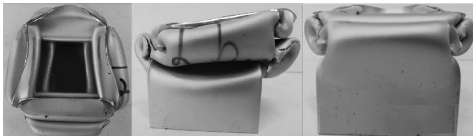
Figure 57 Final views of crushed specimen in test 2b under contact in edge
