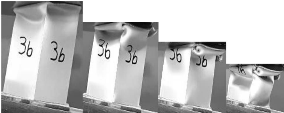
Figure 73 Collapse states of test 3b under contact in corner
