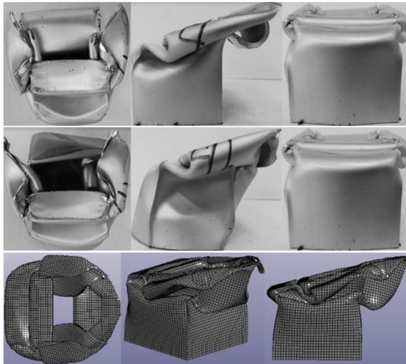
Figure 170 Collapsed structures for case 4-edge (top: test 4a, mid: test 4b, bottom: LS DYNA)
