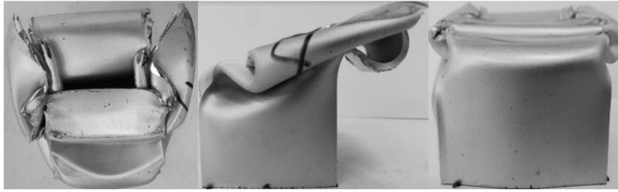
Figure 80 Final views of crushed specimen in test 4a under contact in edge
