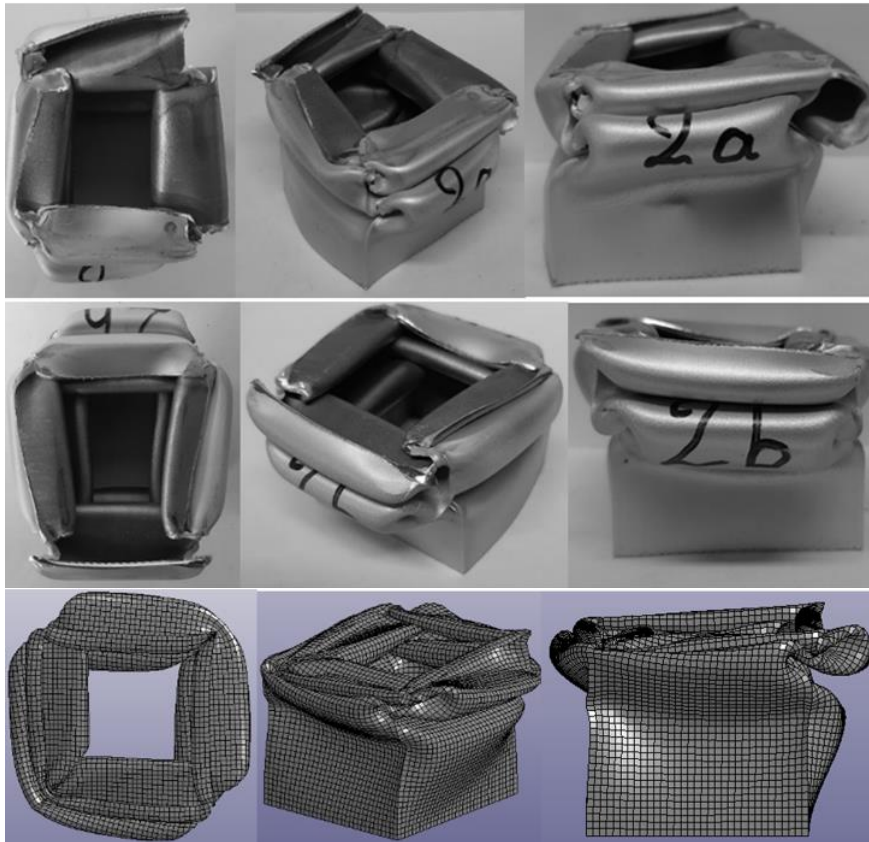
Figure 161 Collapsed structures for case 2-corner (top: test 2a, mid: test 2b, bottom: LS DYNA)
