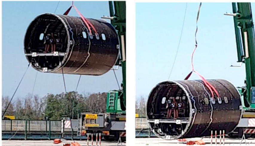
Figure 26 Impact crush test of aircraft's fuselage, [8]
