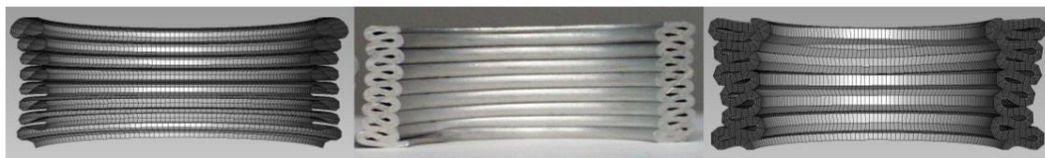
Figure 27 Bare tube folds prediction (shell elements model, experimental specimen, solid elements model), [13]
