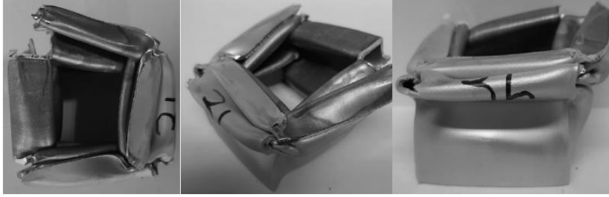
Figure 75 Final views of crushed specimen in test 3b under contact in corner
