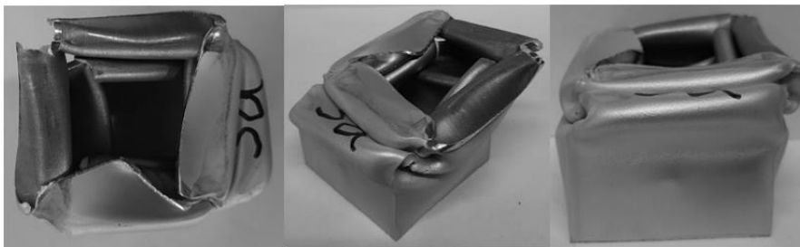
Figure 74 Final views of crushed specimen in test 3a under contact in corner
