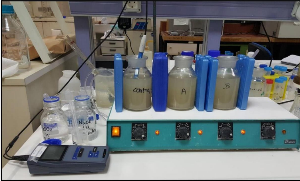
Figure 4.5. Samples during the anoxic phase of a typical experiment investigating anoxic PUR. At this instance, ice packs have been applied to the reactors to keep temperature within the desired range.
