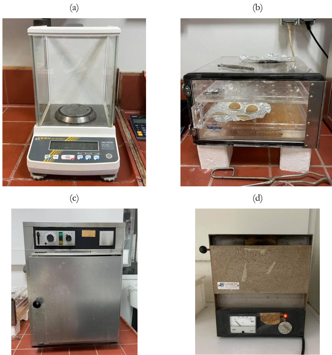
Figure 4.9. Appliances for TSS and VSS analysis. (a): precision scale, (b): dryer, (c): evaporation oven, d): combustion oven
